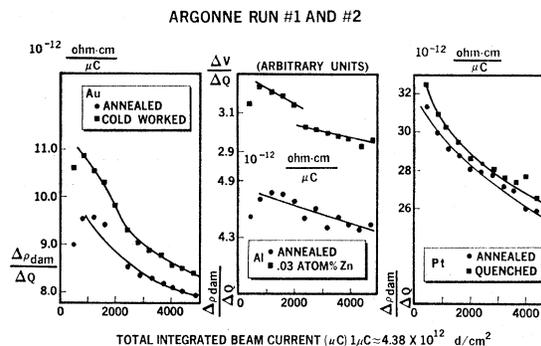
FIG. 2. The damage rates for the six specimens used in Argonne Runs Nos. 1 and 2 are plotted versus the total dose.  $1 \mu\text{C}$  corresponds to approximately  $4.38 \times 10^{12} \text{ d/cm}^2$ . For apparent radiation annealing in the aluminum specimens see main text.
