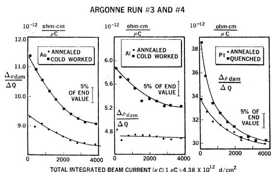
FIG. 1. The damage rates for the six specimens in Argonne Runs Nos. 3 and 4.  $1 \mu\text{C}$  corresponds to approximately  $4.38 \times 10^{12} \text{ d/cm}^2$ . To help visualize the decrease, the magnitude of 5% of the end value has been indicated.
