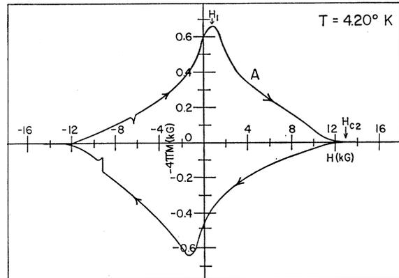
FIG. 7. Isothermal magnetization at  $T = 4.20^\circ\text{K}$  showing the magnetization of sample A as a function of external magnetic field  $H$  (kG) for both increasing and decreasing field using the dynamic method. The kinks in the curve are caused by flux jumps.
