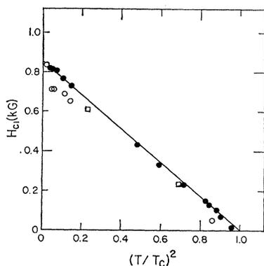
FIG. 5. Plot of  $H_{c1}$  (kG) versus  $(T/T_c)^2$  for samples U and A using flip-coil and dynamic method as follows: solid circle—sample U (flip-coil method); open circle—sample U (dynamic method); open square—sample A (dynamic method).
