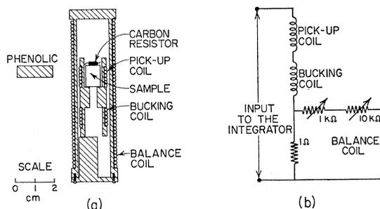
FIG. 2. (a) Diagram of sample and search coils used in the dynamic method. (b) Circuit showing search-coil connections.
