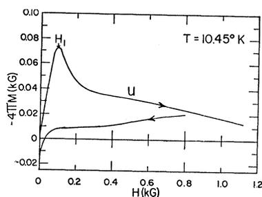
FIG. 3. Typical magnetization curve for sample U taken at  $T=10.45^\circ\text{K}$  with the flip-coil method.
