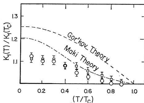
FIG. 8. Plot of our estimations of  $\kappa_1(T)/\kappa_1(T_c)$  versus  $T/T_c$ . (Points: open circle—sample U; open square—sample A.) Dashed curve shows theoretical evaluation by Gor'kov (Ref. 18); dashed and dotted curve shows theoretical evaluation by Maki (Ref. 12).
