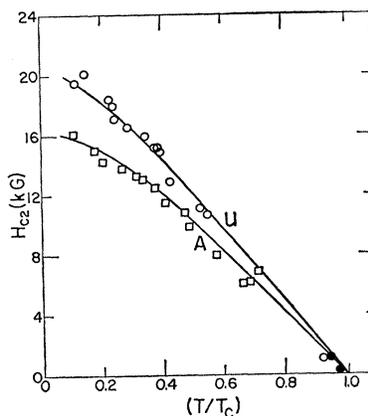
FIG. 6. Plot of observed values of  $H_{c2}$  (kG) versus  $(T/T_c)^2$  for samples U and A as follows: solid circle—sample U (flip-coil method); open circle—sample U (dynamic method); open square—sample A (dynamic method).
