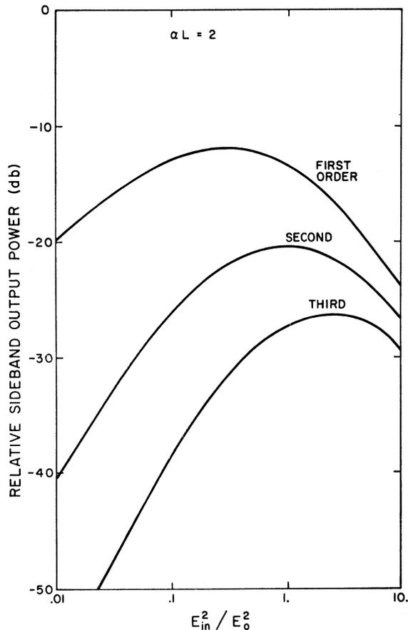
FIG. 6. Relative output sideband power as a function of field strength.
