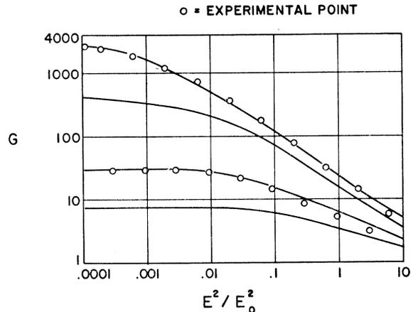
FIG. 3. Integrated gain saturation, compared with experiment.
