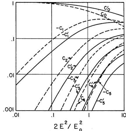
FIG. 5. Fourier gain modulation coefficients for the inhomogeneous line.
