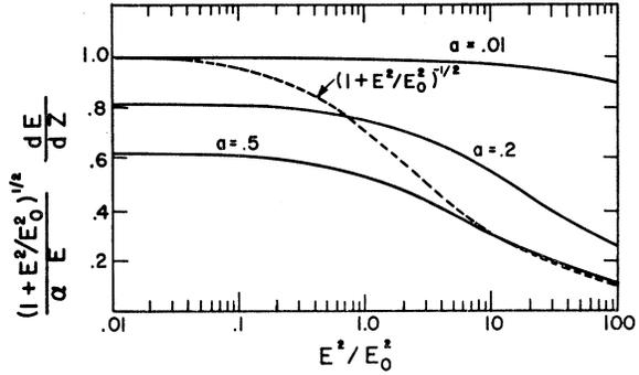
FIG. 2. Gain saturation as a function of field strength, compared to homogeneous gain saturation.
