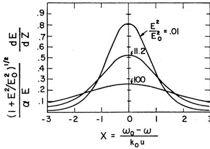
FIG. 1. Gain saturation and broadening as a function of frequency for  $a=0.2$ .
