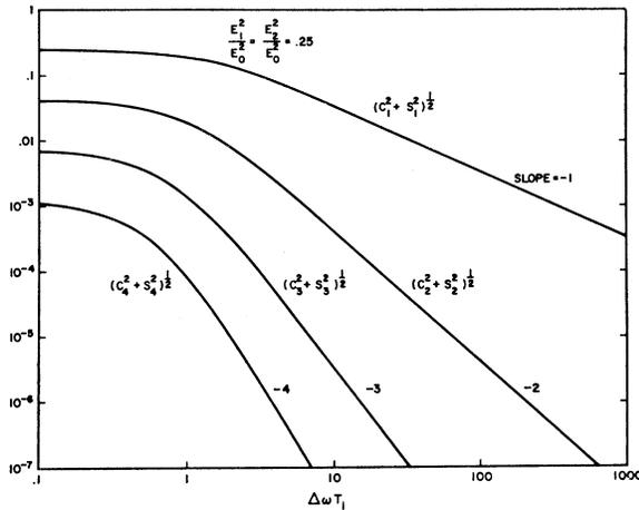
FIG. 7. Fourier gain modulation coefficients as a function of frequency spacing of inducing fields.
