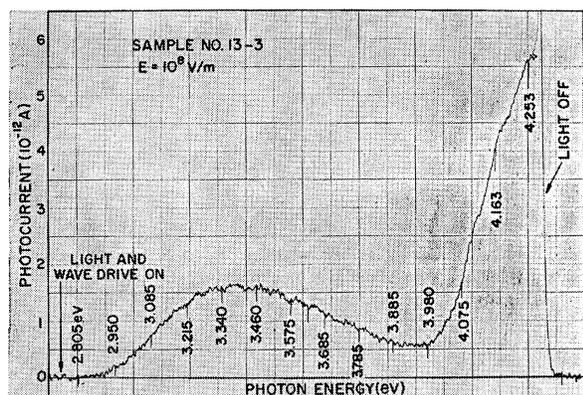
FIG. 1. Photocurrent versus photon energy for sample 13-3. The electric field in the oxide is  $10^8$  V/m directed toward the silicon.
