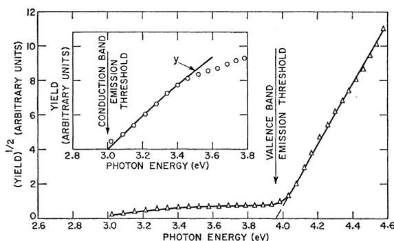
FIG. 2. Square root of yield versus photon energy for sample 13-3. The insert shows a linear plot of yield versus photon energy; the solid curve is a theoretical expression  $y=C[1-(E_0/E)^{1/2}]$  fitted to the experimental points. See text and Appendix for explanation.
