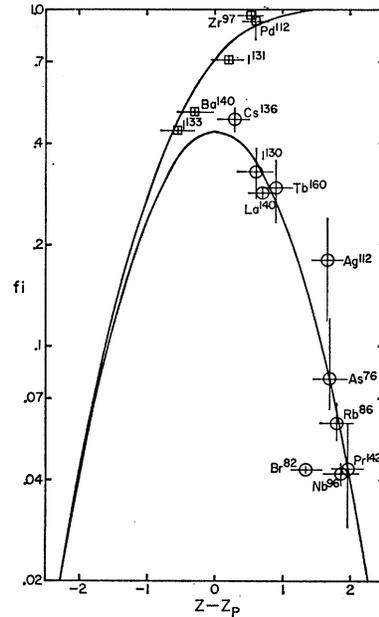
FIG. 4. Gaussian charge distribution for  $\text{Am}^{241*}$  using E.C.D.-G-I (see text). Square symbols refer to cumulative yields.
