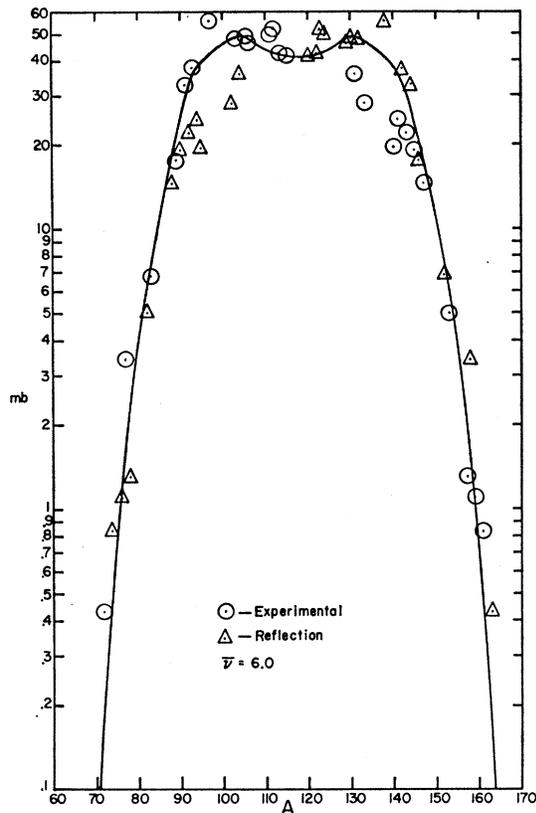
FIG. 8. Apparent mass distribution for the fission of  $\text{Np}^{237}$  induced by 40.5-MeV helium ions. Primary yields were corrected by M.N.P.E.-L-I (see text). The resulting distortion of the yield curve is evident.
