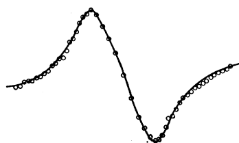
FIG. 12. The \text{Mn}^{55} NMR line-shape data (open circles) compared with a calculated Lorentzian line shape. The value (1/T_2)^{55} = 1.96 \times 10^6 \text{ sec}^{-1} was used in the calculation for the line shape.
