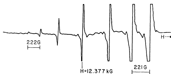
Fig. 2. Spectrum of the seven fine-structure lines of Gd (0.01%) in DyES. The magnetic field is parallel to the c axis. These measurements were made on a 0.86\text{-mm}^3 sphere at 35.49 kMc/sec. The observed intensity distribution results from the low temperature of 1.6^\circ\text{K} . The magnet sweep is nonlinear.
