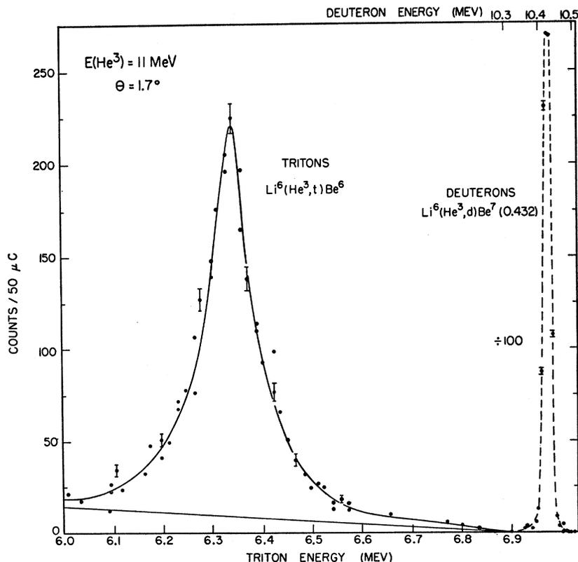
FIG. 1. Momentum spectrum of tritons and deuterons from  $\text{Li}^6 + \text{He}^3$  at  $E_{\text{He}^3} = 11$  MeV. The mean observation angle is  $1.7^\circ$ . The deuteron yield has been divided by 100. The yield at each value of  $B\rho$  has been divided by  $B\rho$  to present a momentum spectrum with constant momentum interval.
