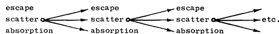
FIG. 2. Each step takes place at a different distance from the surface and hence the probabilities of the three possibilities are different for each step.
