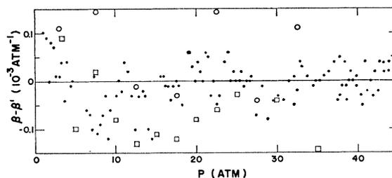
Fig. 3. Deviations of liquid  $\text{He}^4$  compressibility at  $2.200^\circ\text{K}$  from  $0.30 \times 10^{-3} + (72.0 \times 6.66P)^{-1}$ . ● present measurements; ○ derived from density data of Keesom and Keesom (Ref. 1); □ derived from density of Edeskuty and Sherman (Ref. 5).
