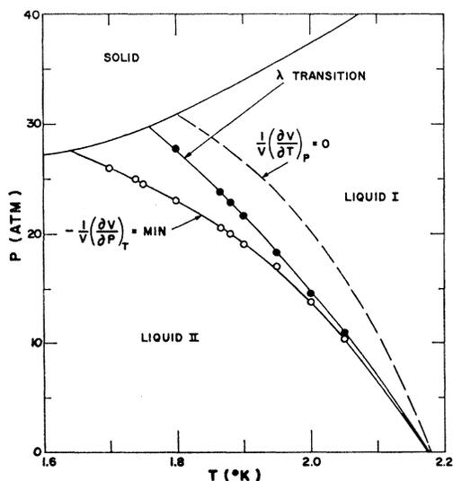
FIG. 7. Phase diagram of He<sup>4</sup> showing the melting curve, the  $\lambda$  line, the locus of zero expansion coefficient, and the locus of minimum in compressibility.
