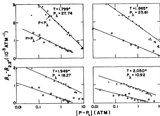
FIG. 8.  $\beta_T - \beta_{2.2}$  versus  $\log|P - P_\lambda|$  for liquid He<sup>4</sup> at several temperatures. The upper curve is for  $P < P_\lambda$  and the lower curve is for  $P > P_\lambda$  at each  $T$ .
