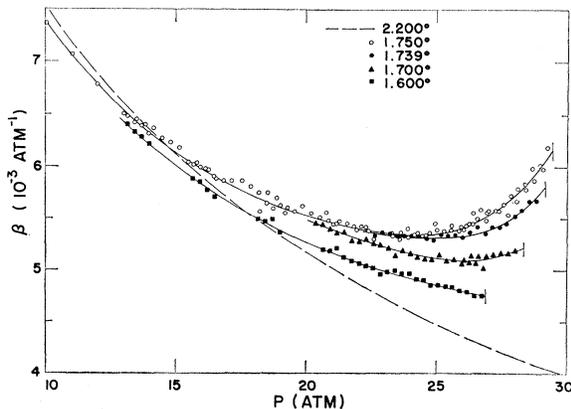
FIG. 6. Compressibility of liquid He<sup>4</sup> at several temperatures below 1.76 and at 2.200°K.
