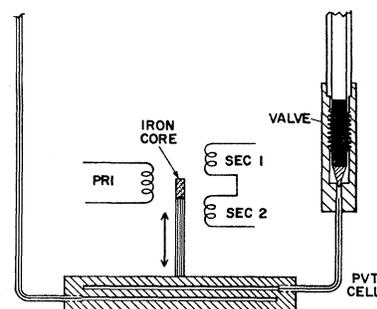
FIG. 1. The  $P$ - $V$ - $T$  cell.
