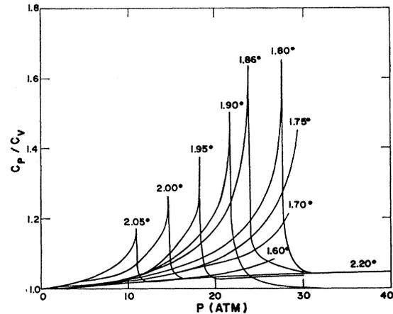
Fig. 9. The ratio of specific heats  $C_P/C_V$  versus pressure for liquid He<sup>4</sup> at several temperatures.
