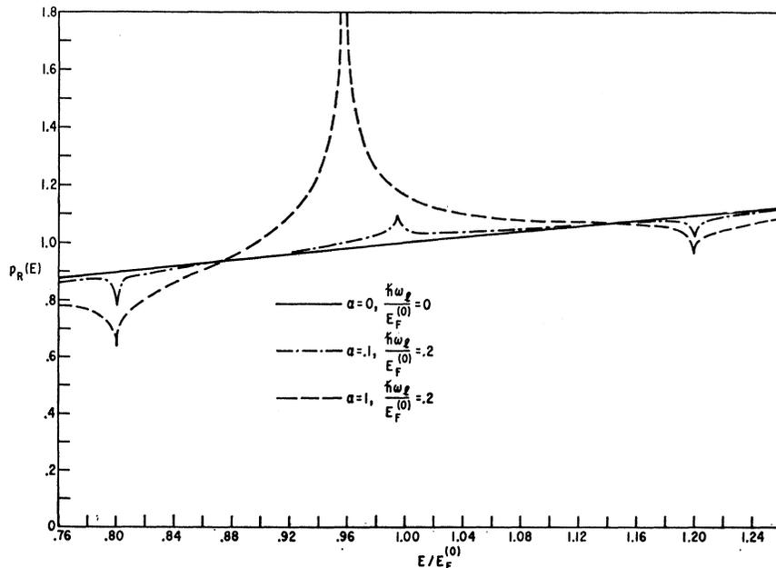
FIG. 2. The reduced electronic density of states  $\rho_R = \pi^2 \hbar \rho / m p_F$  calculated using the unshielded polar interaction between the electrons and longitudinal optical phonons. The introduction of screening eliminates the singularity at  $E = \mu$  but not those at  $E = \mu \pm \omega_0$ . The coupling constants and phonon frequencies are indicated in the figure.
