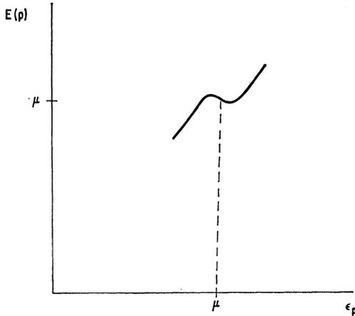
FIG. 1. A schematic representation of the dispersion relation for a polaron when screening is neglected. The extrema near the Fermi energy are exaggerated in the figure. Dielectric screening in the random-phase approximation eliminates this instability.
