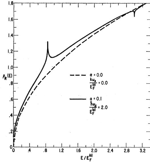
FIG. 3. The reduced electronic density of states  $\rho_R = \pi^2 \hbar \rho / m \dot{p}_F$  calculated using the unshielded polar interaction between the electrons and longitudinal optical phonons. The introduction of screening eliminates the singularity at  $E = \mu$  but not those at  $E = \mu \pm \omega_0$ . The coupling constants and phonon frequencies are indicated in the figure.
