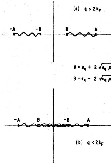
FIG. 6. The cuts of the RPA dielectric function  $\epsilon(q, \omega)$  in  $\omega$  space. The four logarithmic branch points can be connected by two branch cuts. These cuts are distinct for  $q > 2k_F$ , but they overlap for  $q < 2k_F$ . At the point  $\omega = 0$   $\epsilon(q, \omega)$  is analytic because  $\epsilon_r(q, 0) = 0$  for all values of  $q$ .
