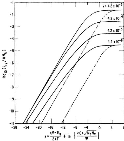
FIG. 3. Plots of the quantity  $J_{rg}/WN_A$ , which is proportional to the recombination-generation current in the depletion region of a diode in which pair recombination predominates. Each curve is labeled with the parameter  $v$ , which is proportional to the majority defect concentration, donors in this case. The solid curves are for the low-temperature regime, the dashed curves for the high-temperature regime.
