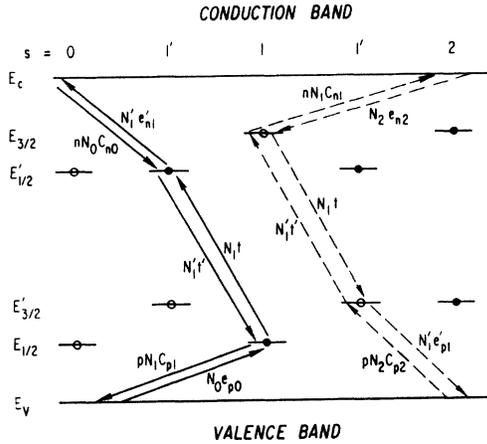
FIG. 1. Energy-level diagram depicting the various transitions giving rise to recombination or generation via a donor-acceptor pair. The unperturbed donor and acceptor levels are  $E_{1/2}'$  and  $E_{3/2}'$  and the perturbed levels are  $E_{1/2}$  and  $E_{3/2}$ , respectively. The  $s$  value denotes the occupancy of the complex,  $s=1'$  meaning the donor is occupied and the acceptor is not.
