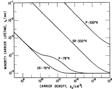
FIG. 2. Low-level minority-carrier lifetime for a hypothetical semiconductor, the characteristics of which are described in the text. The curves labeled P-78°K and P-300°K are for pair recombination at 78 and 300°K, respectively; SR-78°K and SR-300°K are for Shockley-Read statistics at these temperatures.
