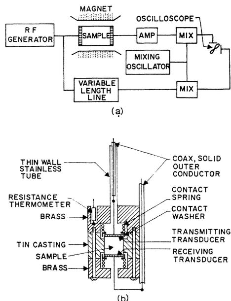
FIG. 1. (a) Block diagram of the experimental apparatus, and, (b) details of the sample holder assembly.
