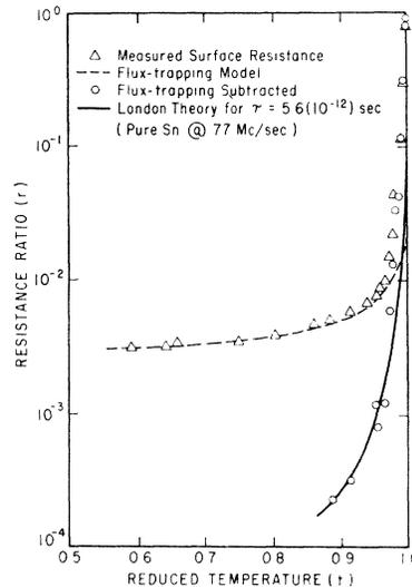
FIG. 6. Plot demonstrating agreement of experimental data with London theory after flux-trapping effect is subtracted.
