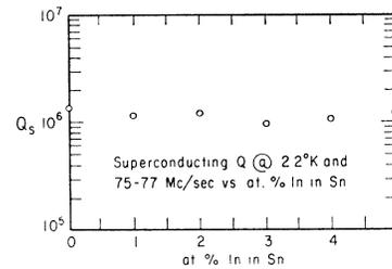
FIG. 2. Superconducting  $Q$  for several circuits plotted against atomic percentage of indium content. Little variation is noted.
