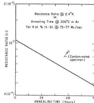
FIG. 3. Plot of resistance ratio at a fixed temperature versus annealing time exhibits an exponential dependence having a characteristic time of 96 h at 200°C.
