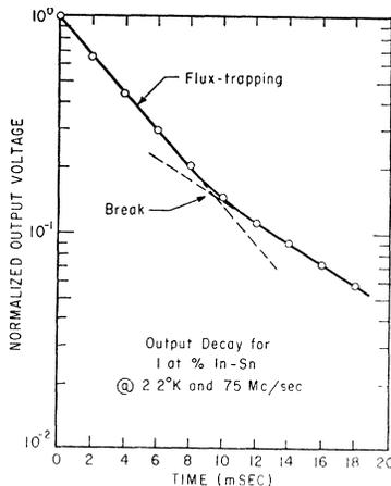
FIG. 5. Plot of decay of normalized output voltage with time, substantiating the existence of a local critical field.
