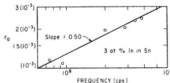
FIG. 1. Residual-resistance ratio plotted versus frequency. The theoretical slope is arbitrarily drawn through the experimental points, showing substantial agreement.
