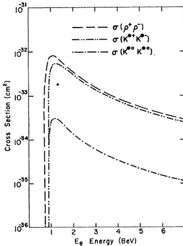
FIG. 4. Total cross sections for  $e^+ + e^- \rightarrow V + V$  processes as a function of the energy of the electron in the center-of-mass system.
