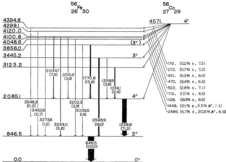
FIG. 5. Decay scheme for  $^{56}\text{Co}$ . Transition energies are given in keV; numbers in parentheses are transition intensities relative to 100 for the 846.5-keV gamma ray. The energies of the positron branches are from Ref. 23.
