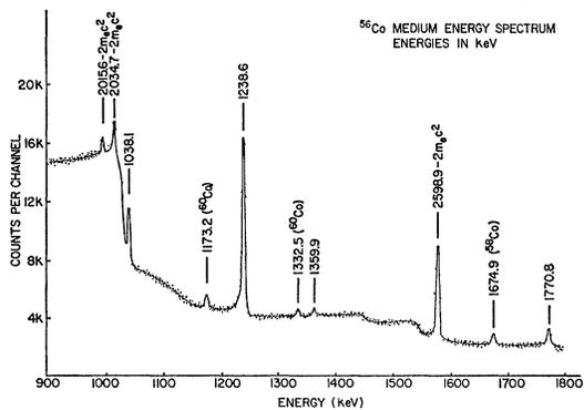
FIG. 3.  $^{56}\text{Co}$  gamma-ray spectrum obtained with a lithium-drifted germanium detector: 900–1800 keV.
