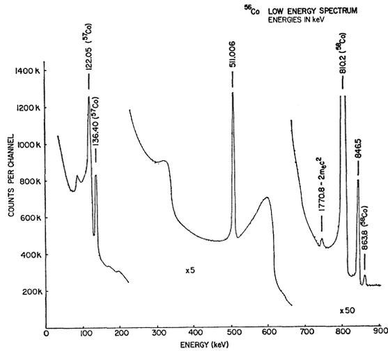
FIG. 2.  $^{56}\text{Co}$  gamma-ray spectrum obtained with a lithium-drifted germanium detector: 0–900 keV.
