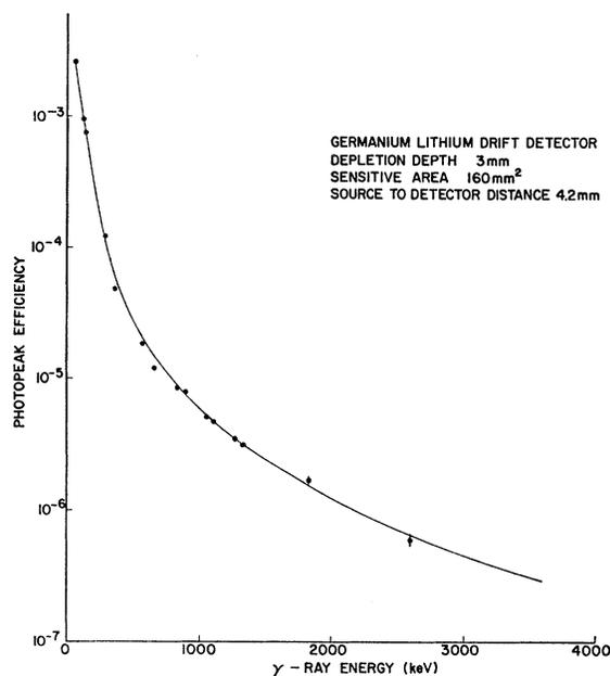
FIG. 1. Efficiency curve for the 3-mm depletion-depth lithium-drifted germanium detector.
