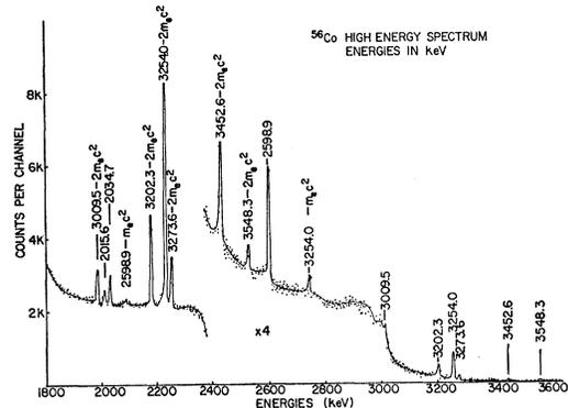
FIG. 4.  $^{56}\text{Co}$  gamma-ray spectrum obtained with a lithium-drifted germanium detector: 1800–3600 keV.
