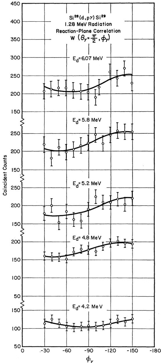
FIG. 6. Reaction plane proton-gamma angular correlations in the de-excitation of the 1.28-MeV state in  $\text{Si}^{29}$ . The geometry is identical with that described in the caption of Fig. 4.
