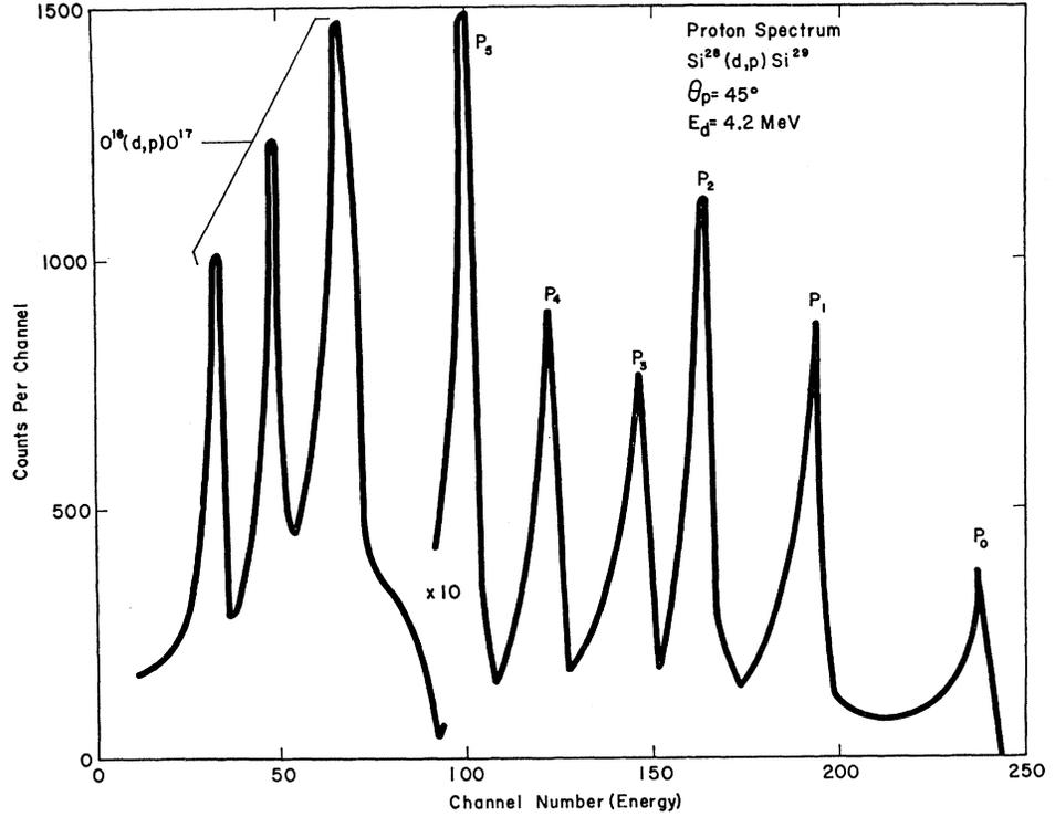
FIG. 1. Part of a spectrum of protons emitted at a laboratory detector angle of  $45^\circ$  in the  $\text{Si}^{28}(d, p)\text{Si}^{29}$  reaction. The peaks labeled  $P_0$ ,  $P_1$ , etc., refer, respectively, to the proton groups which leave  $\text{Si}^{29}$  in its ground, first, etc., excited states.
