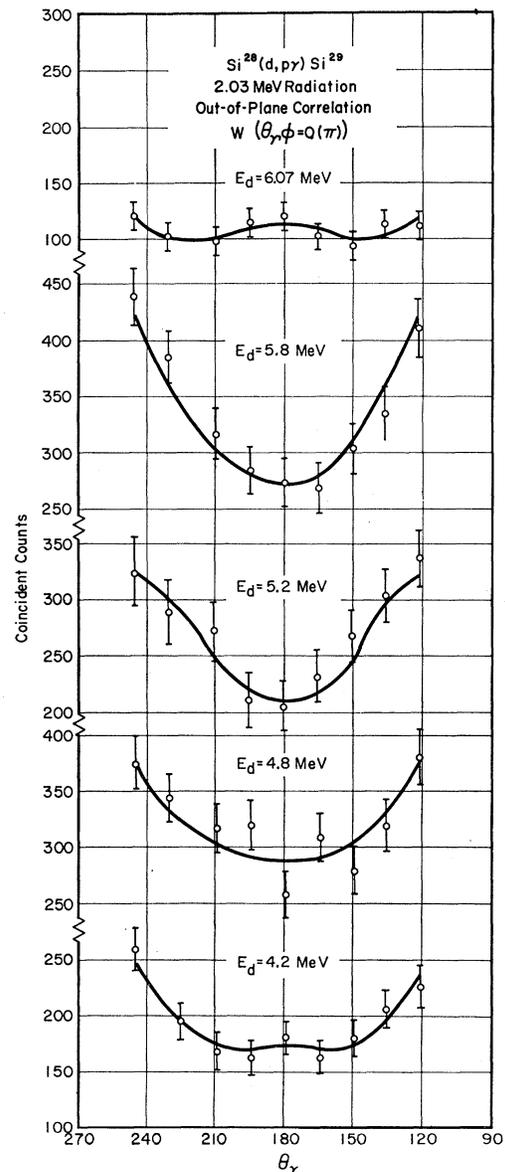
FIG. 5. Proton-gamma angular correlations in the de-excitation of the 2.03-MeV state in  $\text{Si}^{29}$ , measured in that plane perpendicular to the reaction plane which contains the incident beam direction. The geometry used is identical to that described in the caption of Fig. 4.
