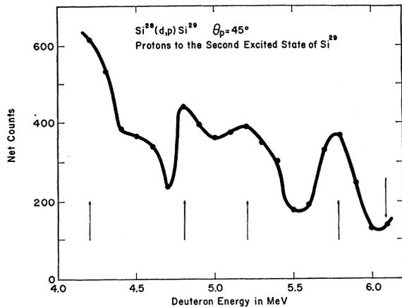
FIG. 3. A thick-target yield curve for the  $P_2$  proton group. The arrows indicate those deuteron bombarding energies at which angular correlations were measured. The solid curve through the experimental points serves only to guide the eye.
