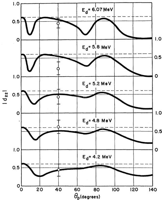
FIG. 11. The solid curves show the calculated values of the magnitude of the normalized statistical tensors  $d_{22}$  as a function of proton detector angle. The solid curves are *not* fits to the experimental data shown. (See caption of Fig. 10.) Plane-wave predictions are shown as dashed curves.
