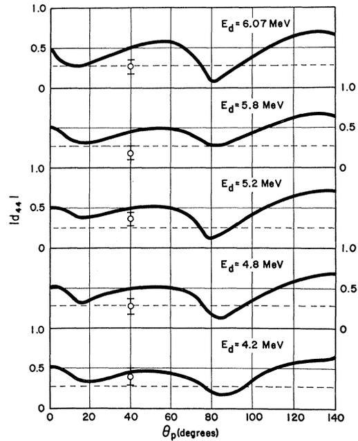
FIG. 12. The solid curves show the calculated values of the magnitude of the normalized statistical tensors  $d_{44}$  as a function of proton detector angle. The solid curves are *not* fits to the experimental data shown. (See caption of Fig. 10.) Plane-wave predictions are shown as dashed curves.
