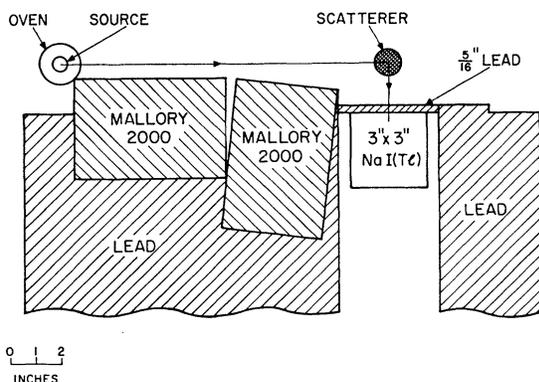
FIG. 2. Typical geometry for the scattering experiment. Of course, the detector was covered with several inches of Pb.
