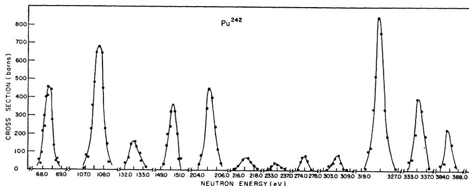
FIG. 3. The resonance cross section from 60 to 400 eV. The solid lines through the points are included to guide the eye. Different abscissa scales are used for the convenience of displaying the data.
