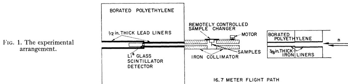
which in turn was located inside a cubic box 3 ft on a side, filled with borated polyethylene pellets. The lead sleeve reduced the intensity of the 480-keV capture  $\gamma$  ray from boron in the neighborhood of the detector. With this geometry, the background as measured by the "thick-absorber" technique was less than 4% over the energy interval investigated.
