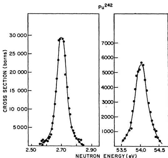
FIG. 2. The resonance cross section below 60 eV. The solid line through the points of the 2.64-eV resonance is a single-level Breit-Wigner fit to the data. The solid line through the 53.5-eV resonance is included to guide the eye.
