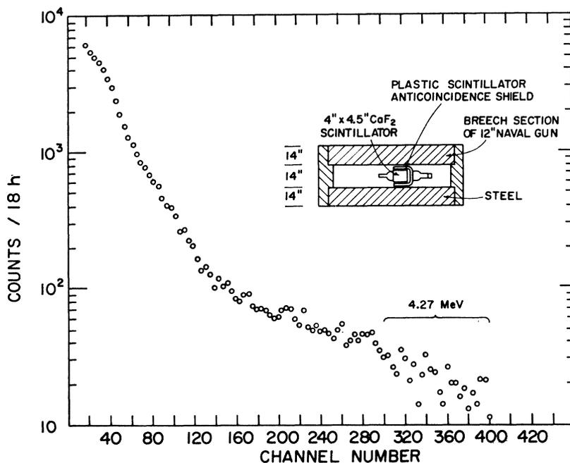
FIG. 2. Search for double beta decay of  $\text{Ca}^{48}$  in single crystal of normal  $\text{CaF}_2$ . Spectrum of counts seen with a 4-in. by 4.5-in. diam. normal  $\text{CaF}_2$  crystal used as a scintillator to detect pulses originating within the crystal. Neutrino-less double beta decay would yield a peak at 4.27 MeV.
