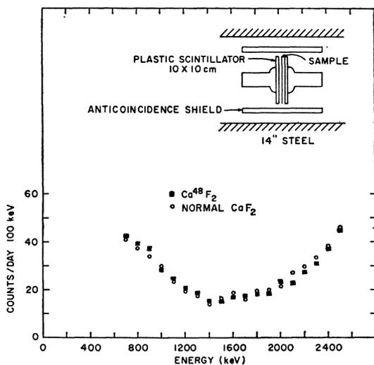
FIG. 6. Spectra of the combined energies of coincidence pulses for  $\text{Ca}^{48}$  and for normal Ca.
