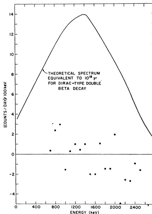
FIG. 7. Difference of the coincidence spectra for  $\text{Ca}^{48}$  and normal Ca of Fig. 6. A theoretical shape for the spectrum of double beta decay with neutrinos is shown which is equivalent to a half-life of  $10^{18}$  yr. This curve is shifted 400 keV to the left to account for self-absorption of the electrons in the sample.
