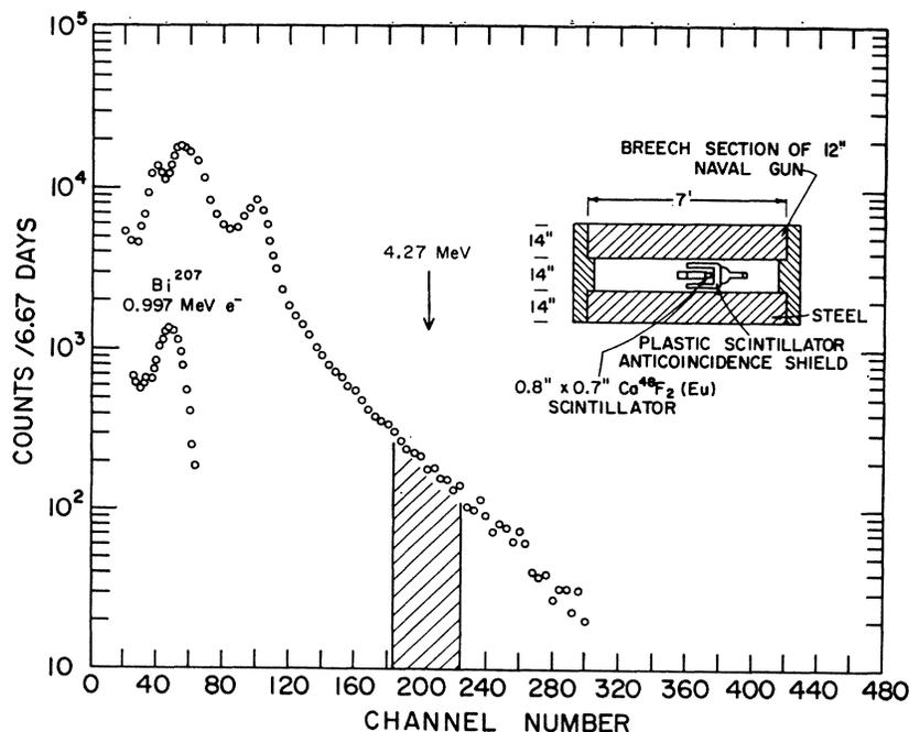
FIG. 3. Spectrum of counts seen with a crystal of  $\text{Ca}^{48}\text{F}_2$  (Eu) enriched to 96.59%  $\text{Ca}^{48}$ . An external source of  $\text{Bi}^{207}$  conversion electrons was used for calibration.
