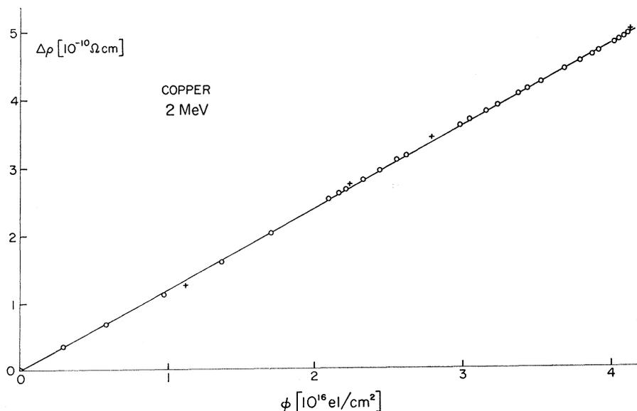
FIG. 1. Production of electrical resistivity in copper as a function of electron dose at 2.0 MeV. The circles are points measured during bombardments and the crosses were measured with the beam off.
