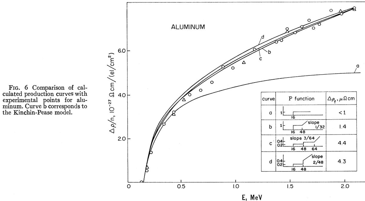
FIG. 6 Comparison of calculated production curves with experimental points for aluminum. Curve b corresponds to the Kinchin-Pease model.
