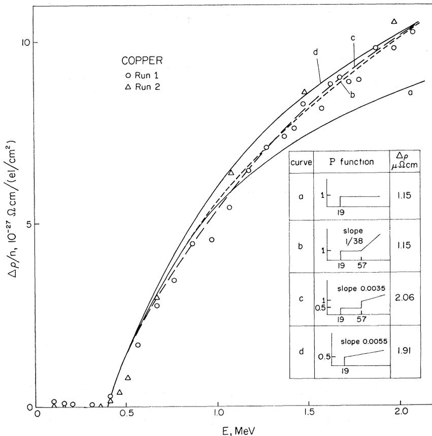
FIG. 5. Comparison of calculated production curves with experimental points for copper. Curve b corresponds to the Kinchin-Pease model.
