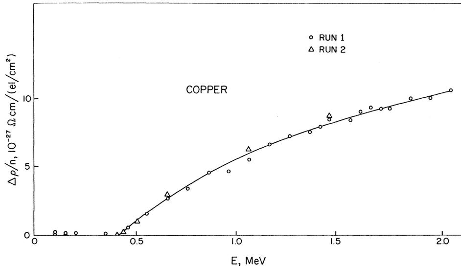
FIG. 3. Rates of electrical resistivity production in copper as a function of electron energy.
