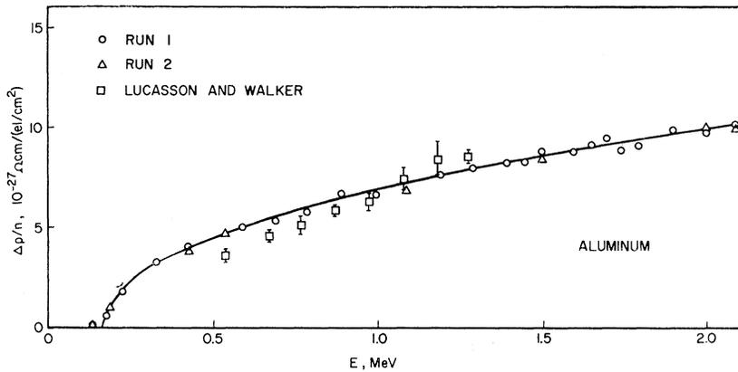
FIG. 4. Rates of electrical resistivity production in aluminum as a function of electron energy.
