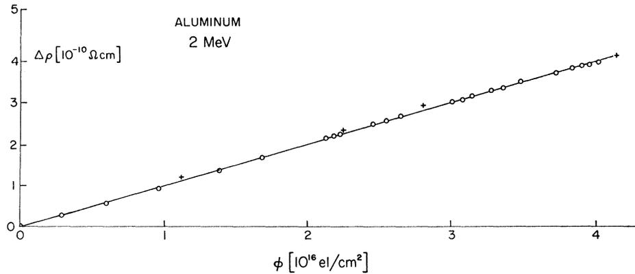
FIG. 2. Production of electrical resistivity in aluminum as a function of electron dose at 2.0 MeV. The circles are points measured during bombardment and the crosses were measured with the beam off.
