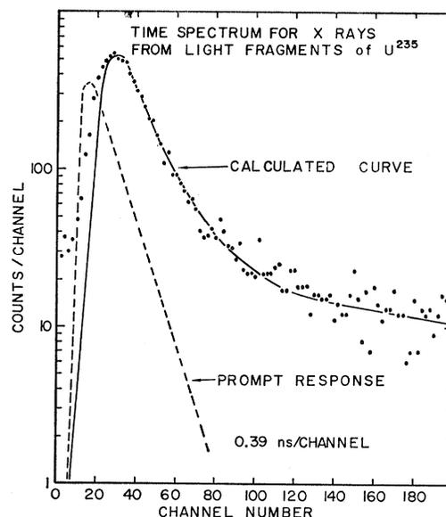
FIG. 6. Time spectrum for light fragment x rays from fission of  $\text{U}^{235}$ . Prompt response was measured by using the  $L$  x ray from  $\text{Th}^{230}$  following alpha decay of  $\text{U}^{234}$ .
