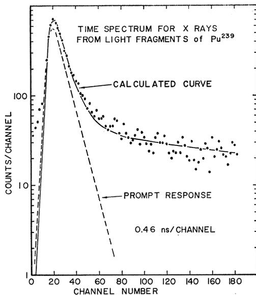
FIG. 4. Time spectrum for light-fragment x rays from fission of  $\text{Pu}^{239}$ . Prompt response was measured by using the  $L$  x ray from  $\text{U}^{235}$  following alpha decay of  $\text{Pu}^{239}$ .
