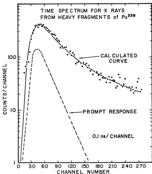
FIG. 5. Time spectrum for heavy fragment x rays from fission of  $\text{Pu}^{239}$ . Prompt response was measured by using internal conversion of  $\text{Cs}^{137}$ .
