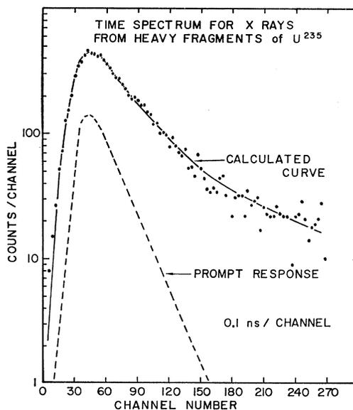
FIG. 7. Time spectrum for heavy-fragment x rays from fission of  $\text{U}^{235}$ . Prompt response was measured by using internal conversion of  $\text{Cs}^{137}$ .
