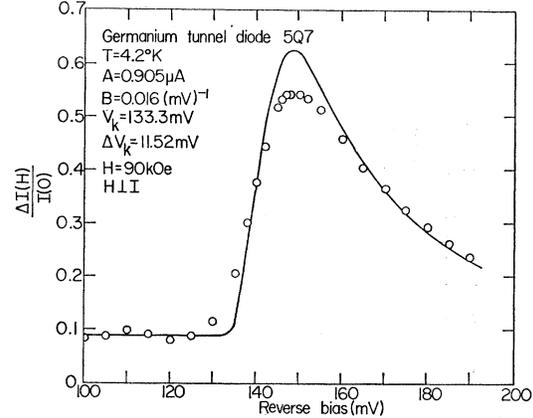
Fig. 10. Relative change of current due to a transverse magnetic field of 90 kOe as a function of reverse bias. The solid curve is obtained using the phenomenological treatment discussed in the text.
