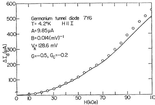
FIG. 6. Magnetic-field dependence of the change in direct tunnel current with  $H \parallel I$  at a bias voltage  $V = 165.8$  mV. The solid curve represents the prediction of Eq. (17).
