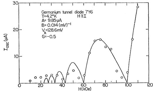
FIG. 7. The oscillatory component of the direct tunnel current as a function of magnetic field with  $H \parallel I$  at a bias voltage  $V = 165.8$  mV. The solid curve represents the prediction of Eq. (22).
