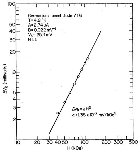
Fig. 9. Magnetic field dependence of  $\Delta V_k$  with  $H \perp I$ .
