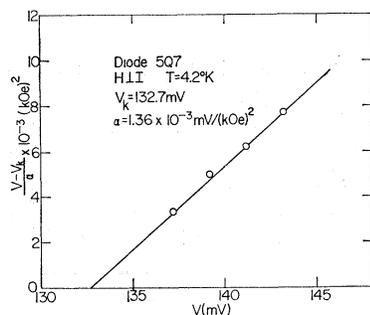
FIG. 12. Graphical determination of  $V_k$  and  $\alpha$  from the data of Fig. 10.
