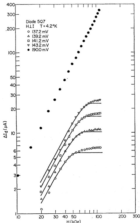
FIG. 11. Magnetic field dependence of the change in direct current at several bias voltages in the vicinity of  $V_k$  with  $H \perp I$ . Shown for comparison is the  $H$  dependence of  $\Delta I$  at  $V = 190$  mV, which does not deviate from its quadratic behavior up to the highest fields studied. The solid lines are theoretical curves based on Eq. (26) in the text.
