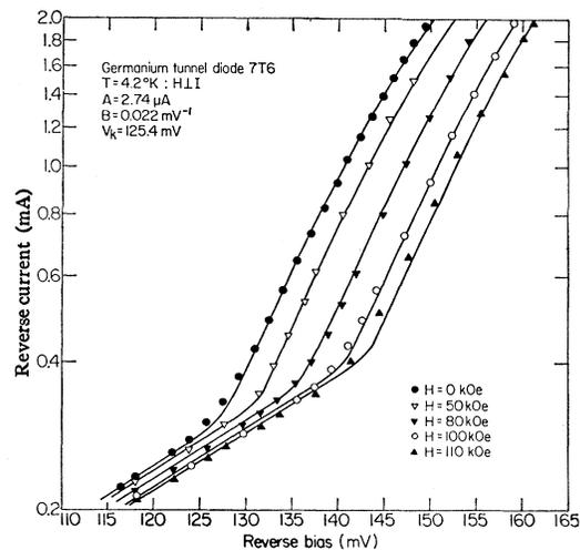
FIG. 8. Current-voltage characteristics of a reverse-biased Sb-doped germanium tunnel diode at  $T = 4.2^\circ\text{K}$  with applied transverse magnetic field as the parameter. The solid curves represent the phenomenological theory discussed in the text.
