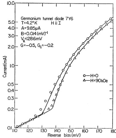
FIG. 4. Current-voltage characteristics of a reverse-biased Sb-doped germanium tunnel diode at 4.2°K with zero magnetic field and with an applied longitudinal field of 90 kOe. The solid curves are the characteristics predicted by the longitudinal theory derived in the text.
