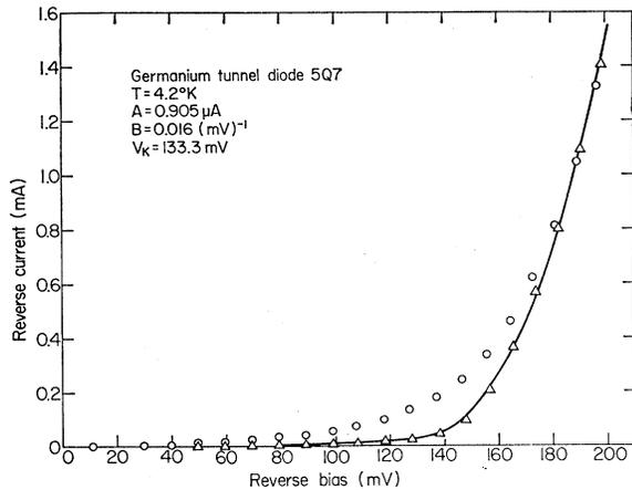
FIG. 2. Reverse current-voltage characteristic of a typical Sb-doped germanium tunnel diode at 4.2°K. The circles show the characteristic of the same diode at 300°K. The solid line shows the theoretical fit to the 4.2°K characteristic.
