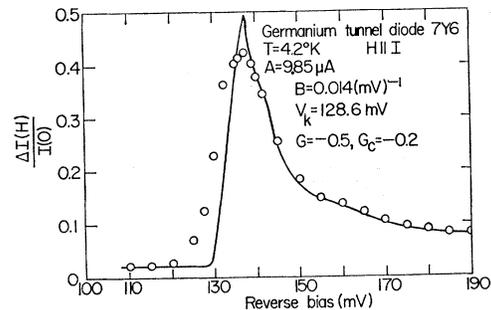
FIG. 5. Relative change of current due to a longitudinal magnetic field of 90 kOe as a function of reverse bias. The solid curve shows the theoretical fit to the data.
