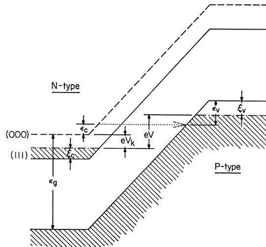
FIG. 3. Potential-energy diagram of a reverse-biased germanium tunnel diode, indicating the various energies referred to in the text. The dotted line represents a hole tunneling from the [000] conduction-band minimum to the (light-hole) valence band.
