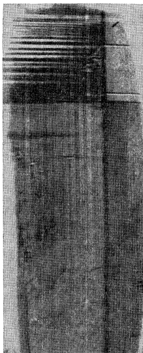
FIG. 3. Example of a Berg-Barrett topograph of V_3Si at 4.7°K. The reflection is 400 with Cu K\alpha radiation. The film plane is normal to the diffracted beam causing a foreshortening in the horizontal direction.
