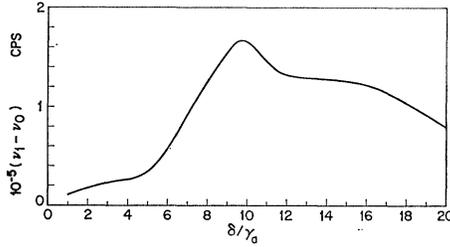
FIG. 7. Beat frequency variation  $\nu_1 - \nu_0$  between  $\pi$  and  $\sigma$  modes with transverse magnetic field. Laser detuning  $\omega_0 - \nu_n = 8\gamma_a$ ;  $\eta = 2$ ;  $\nu/Q = 10^6$ .
