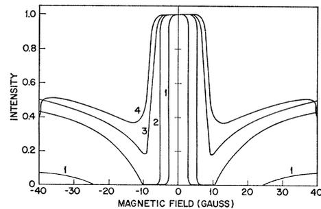
FIG. 14. Variation of  $\pi$  mode intensity with transverse magnetic field. Laser tuning  $\Delta f = (\omega_0 - \nu_n)/2\pi$ . Curve No. 1,  $\Delta f \approx 0$  (in Lamb dip). No. 2,  $\Delta f = 120$ . No. 3,  $\Delta f = 185$ . No. 4,  $\Delta f = 220$  Mc/sec. Rf excitation 9 W. Relative laser intensity 1.9.
