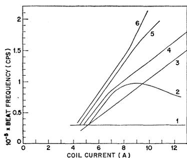
FIG. 16. Experimental curves of beat frequency versus transverse magnetic field. Curve No. 1. In Lamb dip. No. 2 Laser detuning  $\Delta f=150$ , No. 3,  $\Delta f=200$ . No. 4,  $\Delta f=250$ . No. 5,  $\Delta f=300$ . No. 6,  $\Delta f=340$  Mc/sec. Transverse magnetic field 11.5 G/A.
