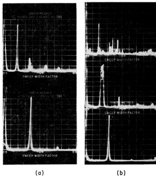
FIG. 17. Beat spectra in the transition between the finite and zero beat frequency regions with transverse magnetic fields. (a) Top trace—Magnetic field 50 G. Bottom trace—Increased to 65 G. (b) Slightly different cavity setting. Magnetic field 39, 41, and 50 G from top to bottom. Spectrum analyzer sweep 20 kc/sec/cm. Zero frequency on left of all traces.
