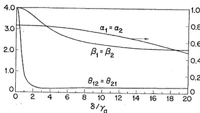
FIG. 8. Variation of the intensity and coupling parameters of the  $\sigma$  modes with axial magnetic field. Laser tuned to line center;  $\eta = 2$ .
