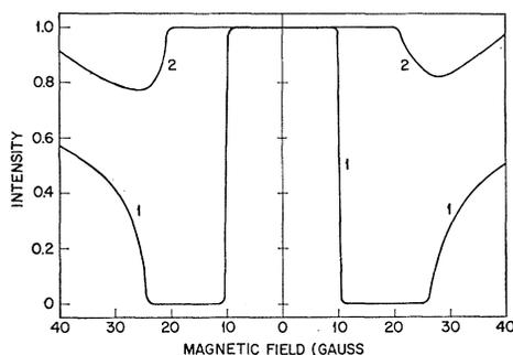
FIG. 15. Variation of  $\pi$  mode intensity with transverse magnetic field. Laser tuning—Curve No. 1, at line center. No. 2,  $\Delta f=235$  Mc/sec. rf excitation 5 W. Relative laser intensity 0.4.
