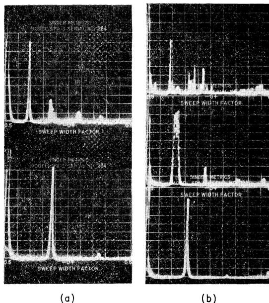
FIG. 17. Beat spectra in the transition between the finite and zero beat frequency regions with transverse magnetic fields. (a) Top trace—Magnetic field 50 G. Bottom trace—Increased to 65 G. (b) Slightly different cavity setting. Magnetic field 39, 41, and 50 G from top to bottom. Spectrum analyzer sweep 20 kc/sec. Zero frequency on left of all traces.
