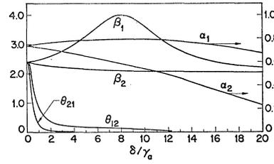
FIG. 9. Variation of the intensity and coupling parameters of the  $\sigma$  modes with axial magnetic field. Laser detuning  $\omega_0 - \nu_n = 8\gamma_a$ ;  $\eta = 2$ .
