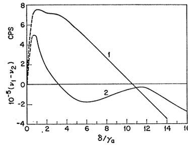
FIG. 13. Beat frequency variation  $\nu_1 - \nu_2$  between the  $\sigma$  modes with axial magnetic field. Curve 1—Laser tuned to line center. Curve 2—Laser detuning  $\omega_0 - \nu_n = 8\gamma_a = 2$ ;  $\nu/Q = 10^6$ .
