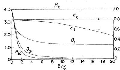
FIG. 2. Variation of the intensity and coupling parameters for  $\pi$  and  $\sigma$  oscillations with transverse magnetic field. Laser tuned to line center;  $\eta_0 = 2$ ,  $\eta_1 = 1.98$ .
