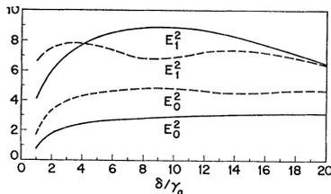
FIG. 5. Intensity parameters  $\pi^{1/2} E^2 |\Delta_0|^2 / (\hbar^2 \gamma_a \gamma_d)$  of the  $\pi$  and  $\sigma$  modes versus transverse magnetic field. Full curves—laser tuned to line center. Dashed curves—laser detuning  $\omega_0 - \nu_n = 8\gamma_a$ .  $\eta_0 = 2$ ,  $\eta_1 = 1.98$ .
