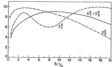
FIG. 10. Intensity parameters  $\pi^{1/2} E^2 |\Delta_1|^2 / (\hbar^2 \gamma_a \gamma_d)$  of the  $\sigma$  modes versus axial magnetic field. Full curve—laser tuned to line center. Dashed curves—laser detuning  $\omega_0 - \nu_n = 8\gamma_a$ ;  $\eta = 2$ .
