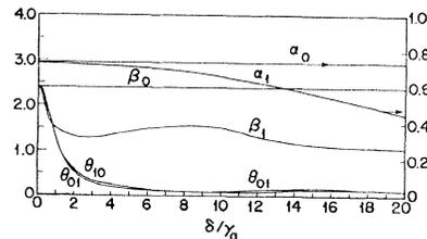
FIG. 4. Variation of the intensity and coupling parameters for  $\pi$  and  $\sigma$  oscillations with transverse magnetic field. Laser detuning  $\omega_0 - \nu_n = 8\gamma_a$ ;  $\eta_0 = 2$ ,  $\eta_1 = 1.98$ .
