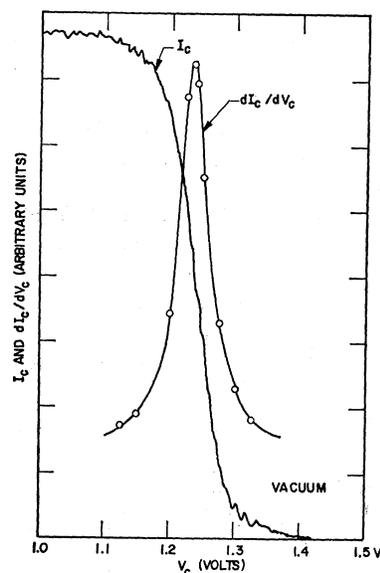
FIG. 2. A typical retarding-potential plot and electron energy distribution obtained therefrom by graphical differentiation.
