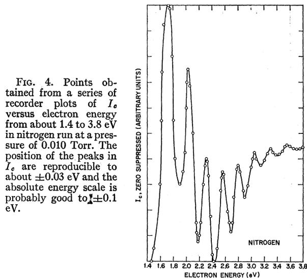
FIG. 4. Points obtained from a series of recorder plots of  $I_c$  versus electron energy from about 1.4 to 3.8 eV in nitrogen run at a pressure of 0.010 Torr. The position of the peaks in  $I_c$  are reproducible to about  $\pm 0.03$  eV and the absolute energy scale is probably good to  $\pm 0.1$  eV.
