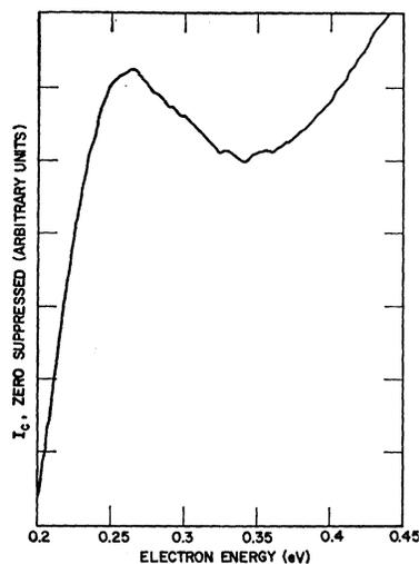
FIG. 5. A recorder tracing of  $I_c$  versus electron energy from 0.2 to 0.45 eV in nitrogen run at a pressure of 0.02 Torr. This plot shows a false "resonance" at about 0.26 eV.
