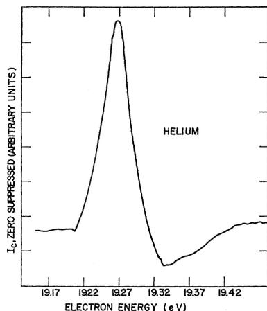
FIG. 3. A recorder tracing of  $I_c$  versus electron energy in the vicinity of the strong helium resonance at 19.27 eV run at a pressure of 0.040 Torr.
