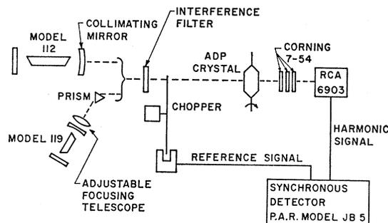
FIG. 1. Harmonic-generating experiment.
