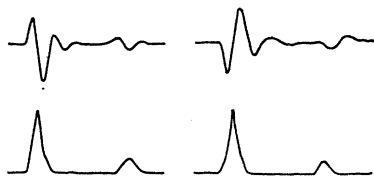
FIG. 2. Typical IFE signals observed in \text{Eu}^{2+} : \text{CaF}_2 at 4.2°K. The signals are on top and the laser power is shown below. On the left is the signal for left circularly polarized light and on the right for right circularly polarized light.
