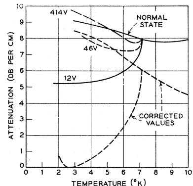
FIG. 1. Attenuation in lead single crystal for longitudinal waves at 50 Mc/sec as a function of the temperature and voltage applied to the transducer (after Love, Shaw, and Fate).
