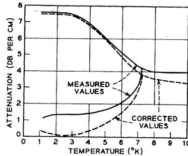
FIG. 7. Measurements of Tittmann and Bömmel and corrections for dislocation damping.
