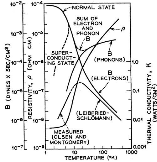
FIG. 2. Drag coefficients for electron damping in the normal and superconducting ranges. Other curves show resistivity of lead and phonon damping of dislocations calculated from the thermal conductivity curve shown.
