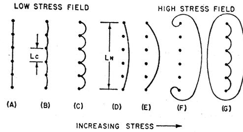
FIG. 4. Dislocation processes occurring at various stress amplitudes (after Granato and Lücke).
