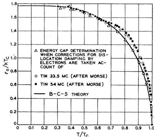
FIG. 8. Comparison of drop in attenuation in the superconducting range with that predicted from BCS theory. Triangles show effect of taking account of dislocation damping.
