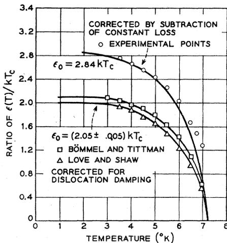
FIG. 6. Evaluation of energy gap taking account of dislocation damping corrections. Top curve shows effect of subtracting a constant loss from both normal and superconducting states.
