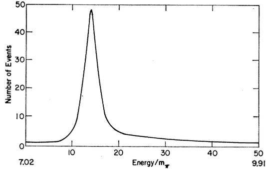
FIG. 9.  $K^+K^-\pi^-$  final state:  $K^+\pi^-$  total energy spectrum for both kinds of vertex. No  $\phi$  peak appears in the  $K^+K^-$  spectrum.
