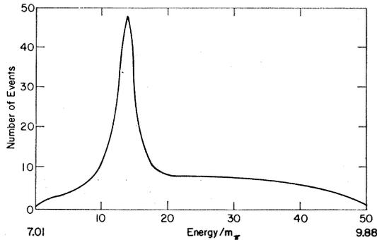
FIG. 8.  $K^-\pi^0 K^0$  final state:  $K^-\pi^0$  or  $K^0\pi^0$  total energy spectrum for both kinds of vertex.
