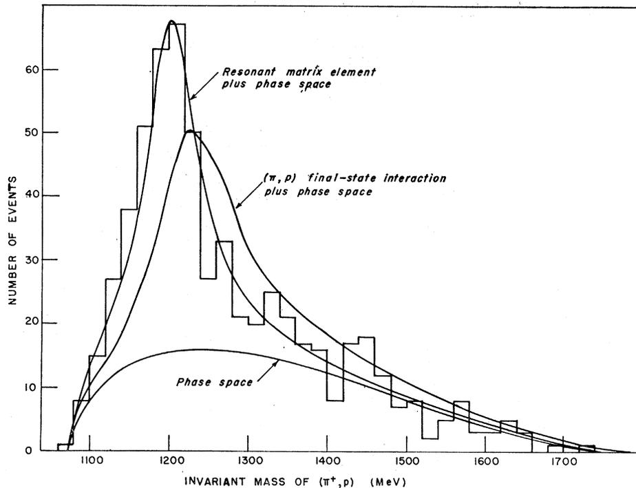
FIG. 1. The  $(\pi^+, p)$  invariant-mass distribution in the reaction  $\pi^- + p \rightarrow \pi^- + \pi^+ + \pi^- + p$ . Shown as solid curves are: (a) the phase-space distribution, (b) phase space plus a Breit-Wigner resonance (resonant matrix element) and (c) phase space plus final-state  $(\pi^+, p)$  interaction.
