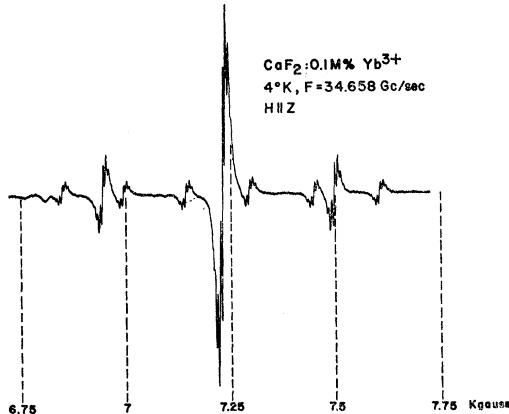
FIG. 8. The EPR spectrum of Yb 3+ in cubic sites in CaF 2 at 35 Gc/sec, 4°K with the external field along a cube axis.
