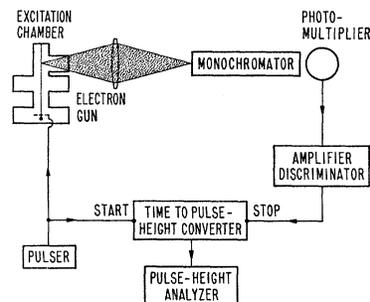
FIG. 1. Block diagram of the experimental setup.
