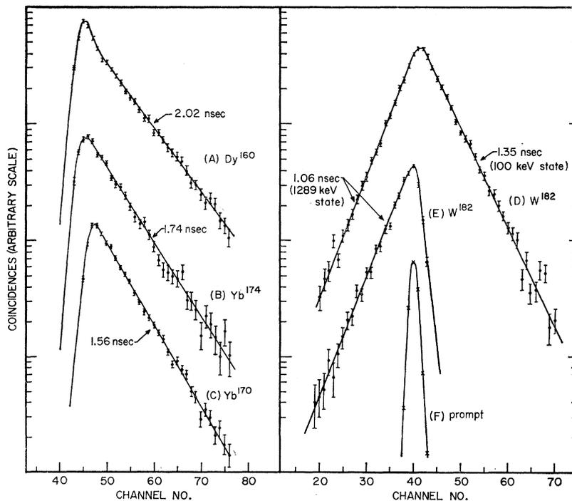
FIG. 3. Half-life curves obtained for the first  $2+$  states in  $Dy^{160}$ ,  $Yb^{174}$ ,  $Yb^{170}$ ,  $W^{182}$ , and the 1289-keV state in  $W^{182}$ . A prompt curve is also shown. Details are given in Table I.
