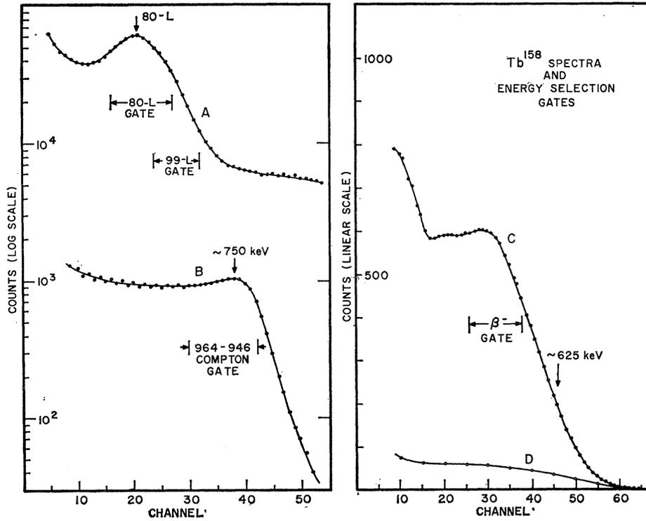
FIG. 2. Curve A shows the  $Tb^{158}$  conversion-electron spectrum observed with the  $\frac{1}{32}$ -in. Pilot B scintillator, curve B the gamma-ray spectrum from the 1-in.  $\times$  1-in. scintillator, curve C the beta spectrum from the  $\frac{1}{16}$ -in. scintillator, and curve D the gamma-ray spectrum from the  $\frac{1}{16}$ -in. scintillator with frontal Al absorber. The energy selection gates are shown for each case.
