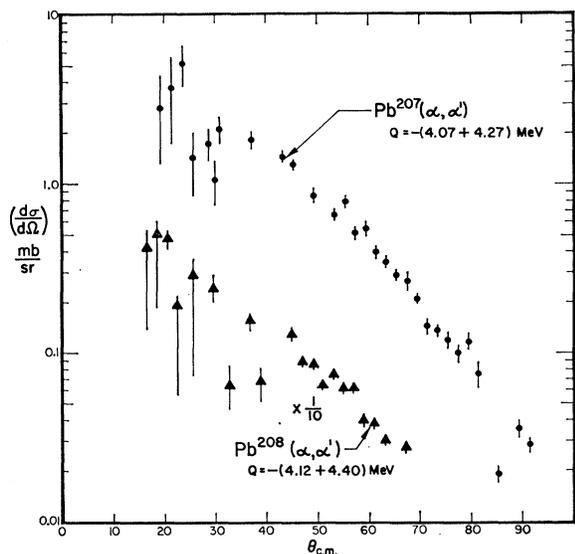
FIG. 7. Angular distribution for the inelastic scattering of 42 MeV  $\alpha$ -particles for the sum of the 4.07- and 4.27-MeV levels in  $\text{Pb}^{207}$  and the sum of the 4.12- and 4.40-MeV levels in  $\text{Pb}^{208}$ .
