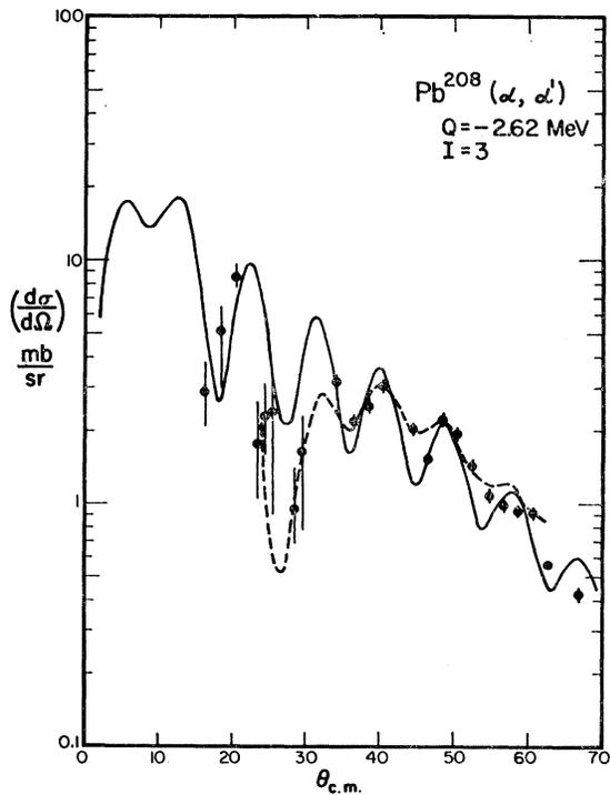
FIG. 4. Angular distribution for the inelastic scattering of 42-MeV  $\alpha$  particles from the 2.615-MeV level in  $Pb^{208}$ . The solid line is the calculated angular distribution calculated with Eq. (1), using the parameter  $l_A=19.7$ ;  $\Delta l_A=0.88$ ,  $\delta=0.25$ ,  $l_s=21.3$ , and  $\Delta l_s=1.05$ . [The dashed line is a DWBA calculation including Coulomb excitation taken from Ref. 9 with  $\beta_2 R=0.88F$ .]
