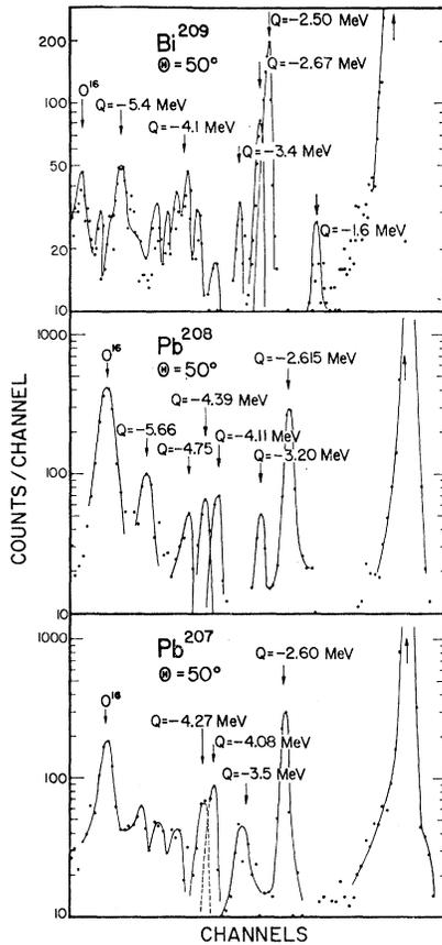
FIG. 1. Energy spectrum of 42-MeV  $\alpha$  particles scattered at 50 deg, for  $Pb^{207}$ ,  $Pb^{208}$ , and  $Bi^{209}$ .
