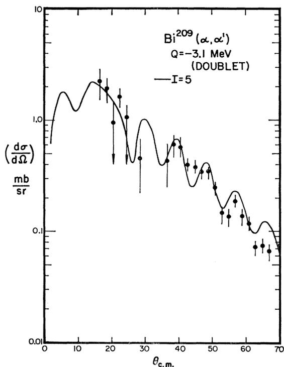
FIG. 5. Angular distribution for the inelastic scattering of 42-MeV  $\alpha$  particles from the doublet at 3.1 MeV in  $\text{Bi}^{209}$ . The solid line is the angular distribution calculated with Eq. (1) for the parameters given in Fig. 4.
