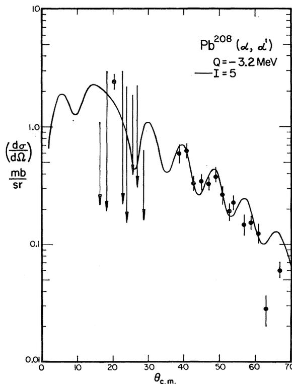
FIG. 6. Angular distribution of the inelastic scattering of 42-MeV  $\alpha$  particles from the 3.198-MeV level in  $\text{Pb}^{208}$ . The solid line is the angular distribution calculated with Eq. (1) using the parameters given in Fig. 4.
