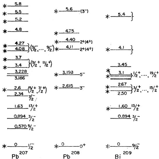
FIG. 2. Level scheme showing the known levels in  $Pb^{207}$ ,  $Pb^{208}$ , and  $Bi^{209}$  below 4 MeV (Refs. 6 and 8) together with all the levels excited in this experiment (preceded by an asterisk). More levels were found by inelastic neutron scattering.
