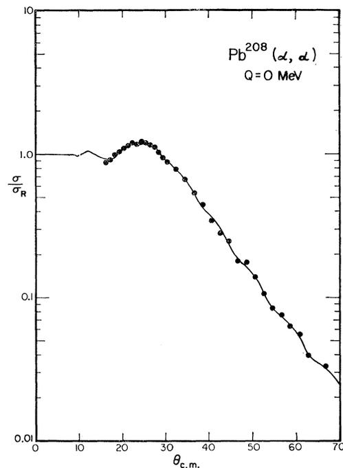
FIG. 10. Angular distribution for the elastic scattering of 42-MeV  $\alpha$  particles divided by Rutherford scattering for Pb<sup>208</sup>. The solid line is the parametrized phase-shift model fitted with the parameters given in Fig. 4.
