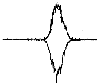
FIG. 2. A tracing of the mass peak wave forms of Fig. 1 here separately amplified and the wave form of (\text{Ba}^{136})^+ inverted. These signals are then presented to the digital memory oscilloscope.
