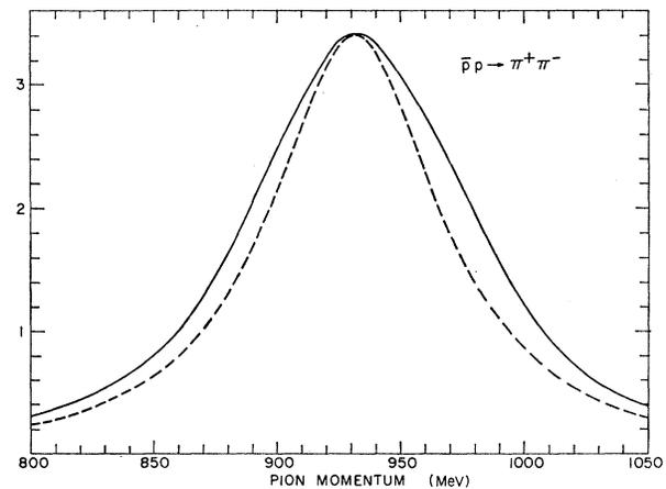
FIG. 2. The solid curve is a Gaussian ideogram of the momentum of 1632 pion tracks from the reaction  $\bar{p}p \rightarrow \pi^+\pi^-$ . The dashed curve is the resolution function for the same events. The vertical scale is in arbitrary units.
