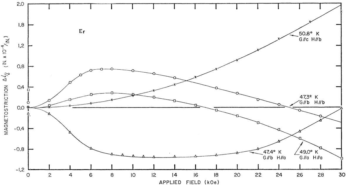
FIG. 5. Magnetostriction of Er as a function of applied field in the quasi-antiphase-domain temperature region. The field was applied in the basal plane. G indicates the strain gauge direction.
