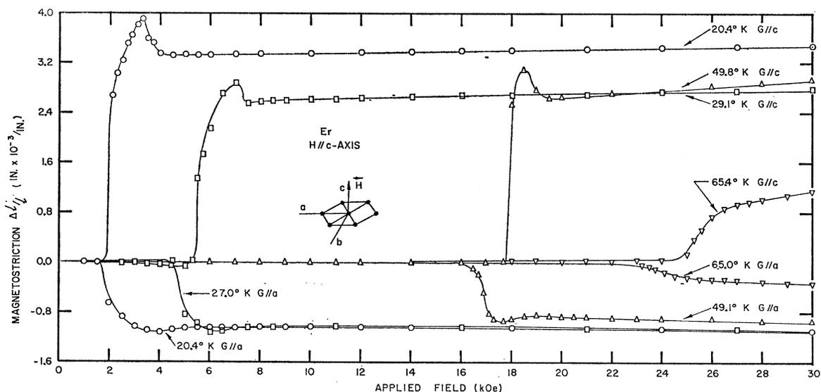
FIG. 2. Magnetostriction of Er as a function of field applied along the  $c$  axis. Temperatures below  $53^\circ\text{K}$  correspond to the quasi-antiphase-domain structure in zero applied field. The  $65^\circ\text{K}$  curves are in the modulated-moment phase. G indicates the strain gauge direction.
