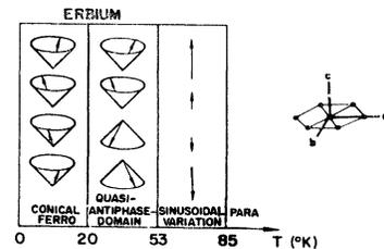
FIG. 1. Magnetic structure of Er in zero applied field observed by neutron diffraction (see Ref. 3).
