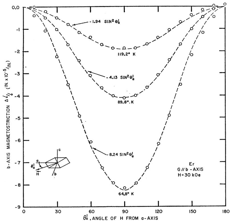
FIG. 8. Second-order theoretical fit and experimental results for the *b*-axis magnetostriction of Er as a function of the applied field angle relative to the *a* axis. The 30-kOe field was applied in the basal plane. At 65°K in zero applied field, Er has the modulated-moment structure. At the other temperatures Er is paramagnetic.
