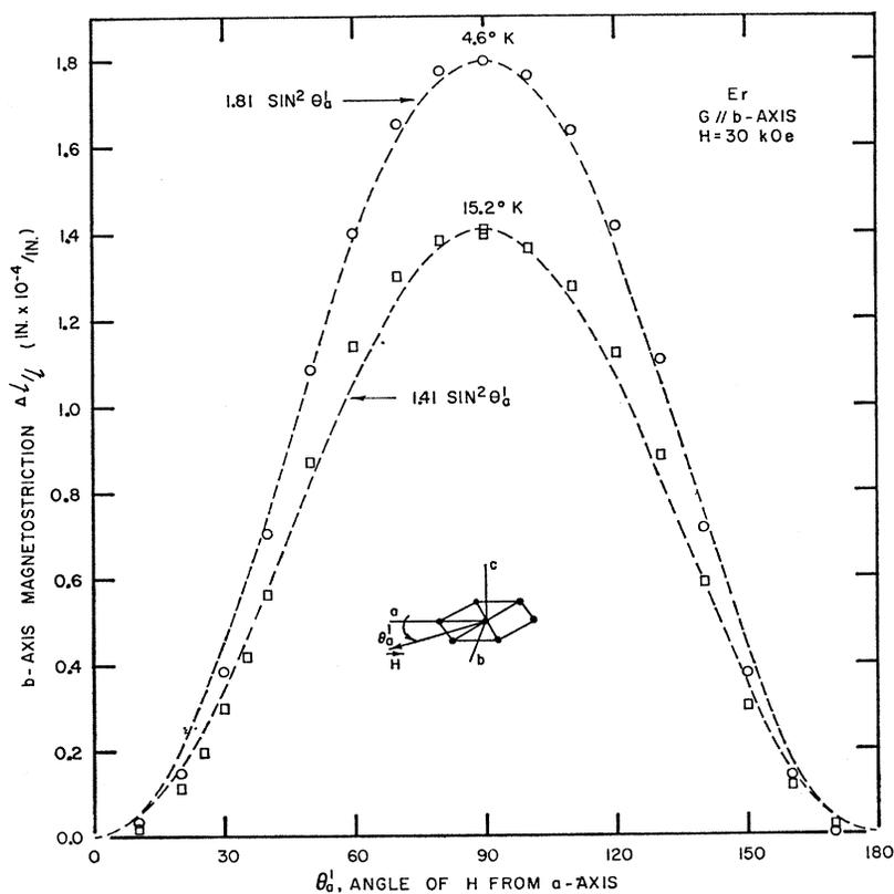
FIG. 9. Second-order theoretical fit and experimental results for the *b*-axis magnetostriction of Er as a function of applied field angle relative to the *a* axis. The 30-kOe field was applied in the basal plane. The zero-external-field state is one of conical ferromagnetism at these temperatures.
