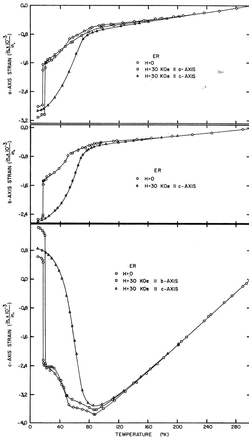
FIG. 10. The *a*-, *b*-, and *c*-axis strain of Er as a function of temperature in zero field and in a 30-kOe field applied along the *c* axis. Results are also given for the *a*- and *c*-axis strains with the field applied in the basal plane.
