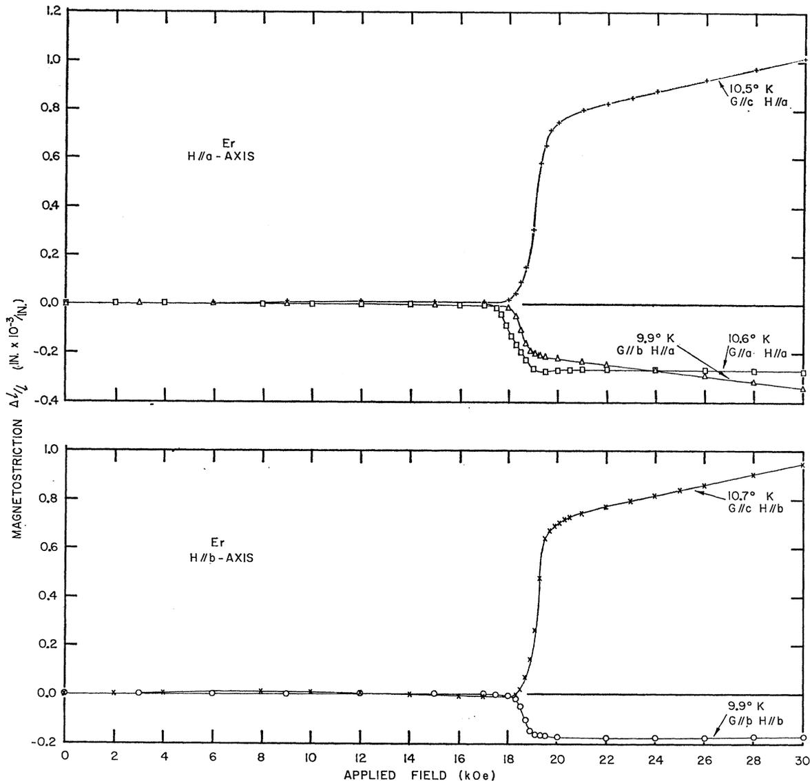
FIG. 3. Magnetostriction of Er as a function of applied field in the conical-ferromagnetic temperature range. The field was applied along the  $a$  axis in the upper figure and along the  $b$  axis in the lower figure.
