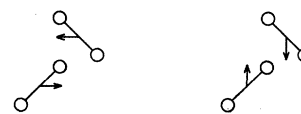
FIG. 6. Translational oscillations of the I_2 molecules as interpreted from far infrared absorption. (Walmsley and Anderson).
