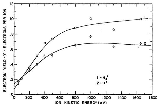
FIG. 8. Electron-yield variation with kinetic energy for  $H^+$  and  $H_2^+$  from gas-covered surface of Mo.
