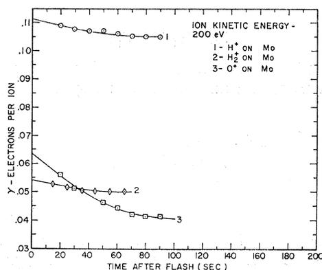
Fig. 1. Variation of secondary electron yield for  $H^+$ ,  $H_2^+$ , and  $O^+$  with time after flash.
