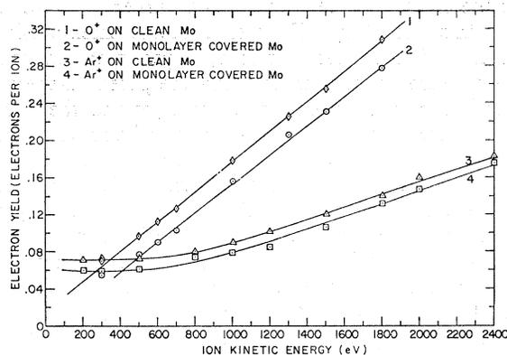
Fig. 2. Electron yields from clean and monolayer-covered surface of Mo bombarded by  $Ar^+$  and  $O^+$ .
