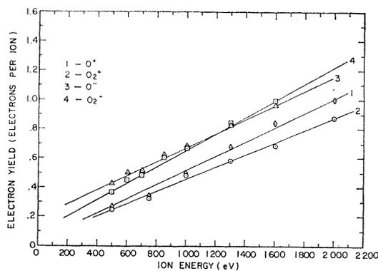
FIG. 6. Variation of  $\gamma$  from an untreated surface of Mo with kinetic energy for  $O^-$ ,  $O_2^-$ ,  $O^+$  and  $O_2^+$  ions.
