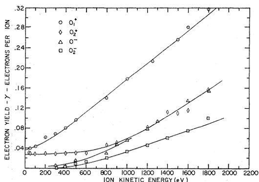
FIG. 3. Electron yields for  $O^+$ ,  $O_2^+$ ,  $O^-$ , and  $O_2^-$  from a clean surface of Mo.
