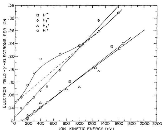
FIG. 5. Electron yields for  $H^+$ ,  $H_2^+$ ,  $H_3^+$ , and  $H^-$  from a clean surface of Mo.
