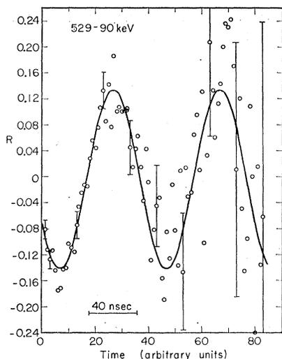
FIG. 5. Measurement of the time-pattern of the angular-correlation precession in an external magnetic field of 41.6 kG using a liquid source. The 529- and 90-keV gamma rays were both detected with  $1\frac{1}{2} \times 1$ -in. NaI(Tl) crystals at a distance of 5 cm. The data shown represent run 6 in Table II.
