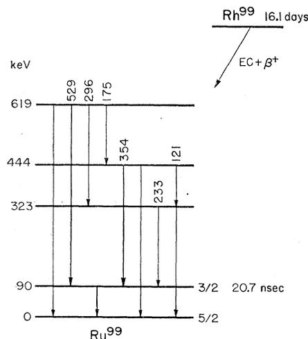
FIG. 2. Lowest part of the  $\text{Ru}^{99}$  decay scheme. The energies have been determined from the  $\gamma$  spectrum shown in Fig. 1.
