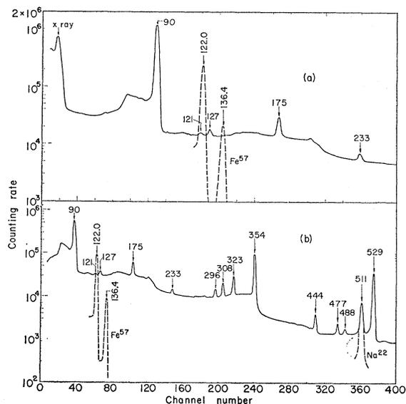
FIG. 1.  $\gamma$ -ray spectrum of the 16-day  $\text{Rh}^{99}$  as recorded with a  $1 \times 2 \text{ cm}^2$  Ge(Li)-detector of 3-mm thickness. The dashed lines are calibration lines.
