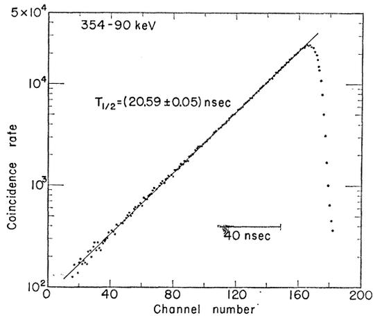
FIG. 3. Half-life measurement of the 90-keV level in  $\text{Ru}^{99}$ . The data shown represent run 2 in Table I.
