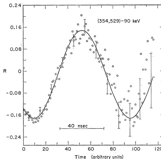
Fig. 6. Measurement of the time-pattern of the angular correlation precession in an external magnetic field of 41.5 kG, using a Ru-Cu alloy source. Both the (529–90)- and the (354–90)-keV cascade were used together in this measurement. The (354,529)- and 90-keV gamma rays were detected with 2- $\times$ -2-in. (distance 7 cm) and 1 $\frac{1}{2}$ - $\times$ -1-in. (distance 5 cm) NaI(Tl) crystals, respectively. The data shown represent run 3 in Table III.
