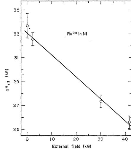
FIG. 7. Measurement of the  $g$  factor and the magnetic hyperfine field of Ru in Ni. The sign of the slope clearly tells that the external magnetic field is opposite to the hyperfine field. The slope of the fitted line yields the  $g$  factor, presuming that magnetic shielding effects are negligible.
