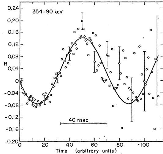
FIG. 4. Measurements of the time-pattern of the angular-correlation precession in an external magnetic field of 41.6 kG using a liquid source. The 354- and 90-keV gamma rays were both detected with  $1\frac{1}{2} \times 1$ -in. NaI(Tl) crystals at a distance of 6 cm. The data shown represent run 2 in Table II.
