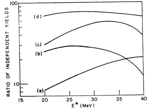
FIG. 8. Ratio of the independent yields (heavy fragment/light fragment). Curve (a), La<sup>140</sup>/Nb<sup>96</sup>; Curve (b), Cs<sup>136</sup>/Y<sup>90</sup>; Curve (c), La<sup>140</sup>/Y<sup>90</sup>; Curve (d), Cs<sup>136</sup>/Nb<sup>96</sup>. The independent yields have been read off the smooth curves in Figs. 3 through 6.
