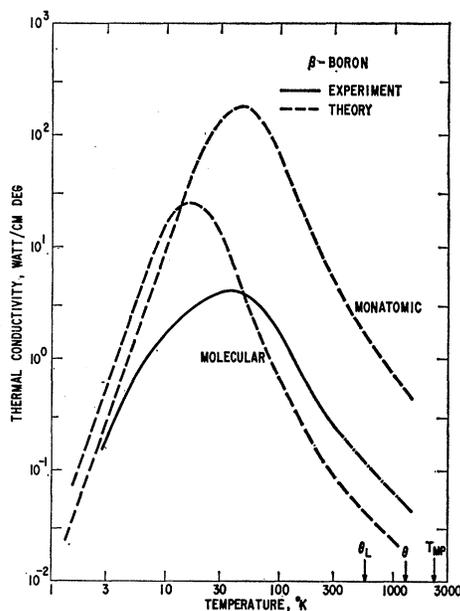
FIG. 5. The thermal conductivity of  $\beta$ -rhombohedral boron versus temperature. The dashed curves show the predicted behavior for boron treated as if it were either a simple molecular solid with a lattice Debye temperature  $\theta_L = 570^\circ\text{K}$  or a simple monatomic solid with a Debye temperature  $\theta = 1300^\circ\text{K}$ . The melting point is  $T_{mp}$ .
