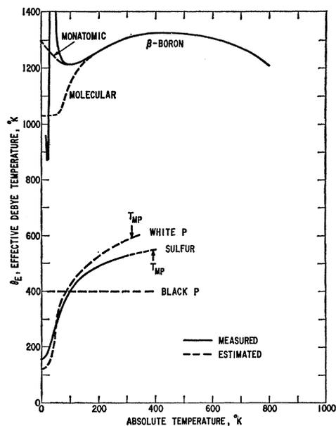
FIG. 4. The effective Debye temperature versus absolute temperature for several solids. This  $\theta_E$  is that value which is calculated from specific heat data when the data are treated as if all of the solids were monatomic. The melting points are *T*<sub>mp</sub>.
