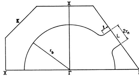
FIG. 1. The model of the Fermi surface used in the calculations to compare with the PRFE and the optical measurements for pure silver and pure gold. The necks consist of a cylindrical section joined smoothly onto a spherical belly. Sections of cross sections in the (100) and (110) planes are shown.
