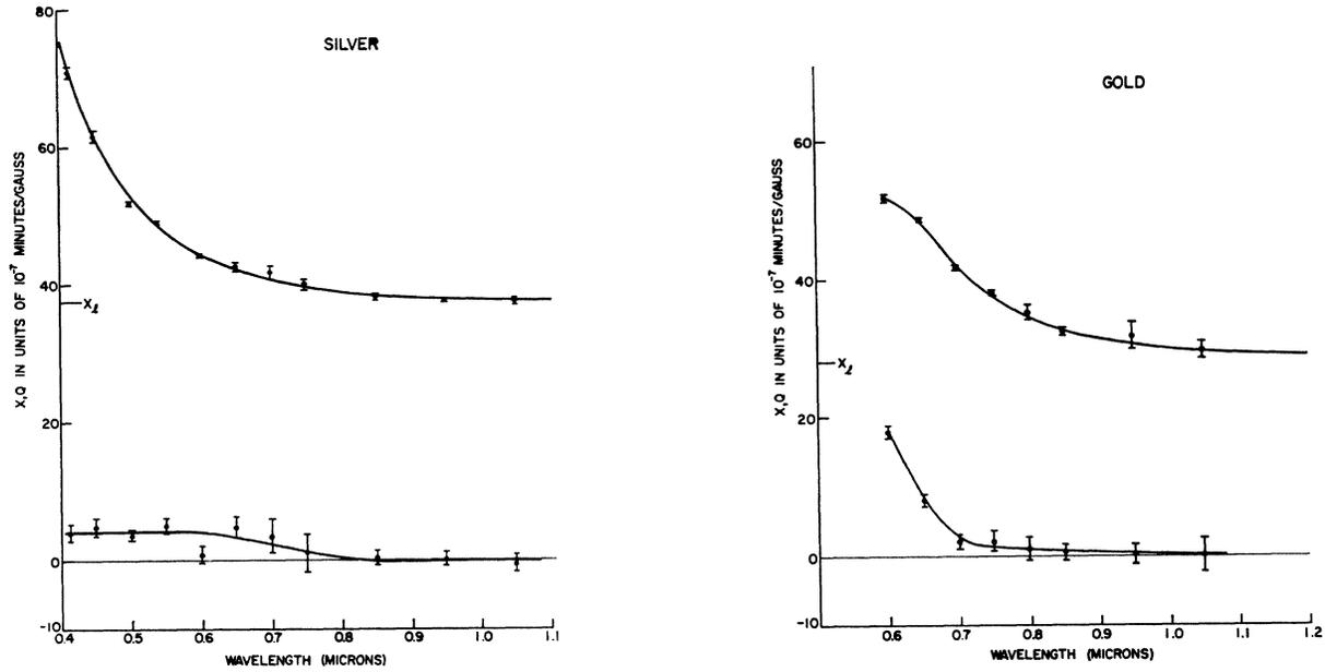
FIG. 4. (a) The values of the measured PRFE angular rotation  $\chi$  and the ellipticity  $Q$  for pure silver as a function of wavelength. The long-wavelength constant value is  $\chi_1$  given in Table I. (b) The values of the measured PRFE angular rotation  $\chi$  and the ellipticity  $Q$  for pure gold as a function of wavelength. The long-wavelength constant value is  $\chi_1$  given in Table I.
