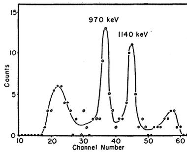
FIG. 6. Spectrum of gamma rays which are in coincidence and sum to form 2110-keV sum peak. The peaks are statistically of equal intensity.
