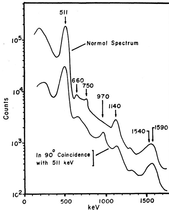
FIG. 7. Spectrum of gamma rays which are in coincidence with 511-keV annihilation radiation.
