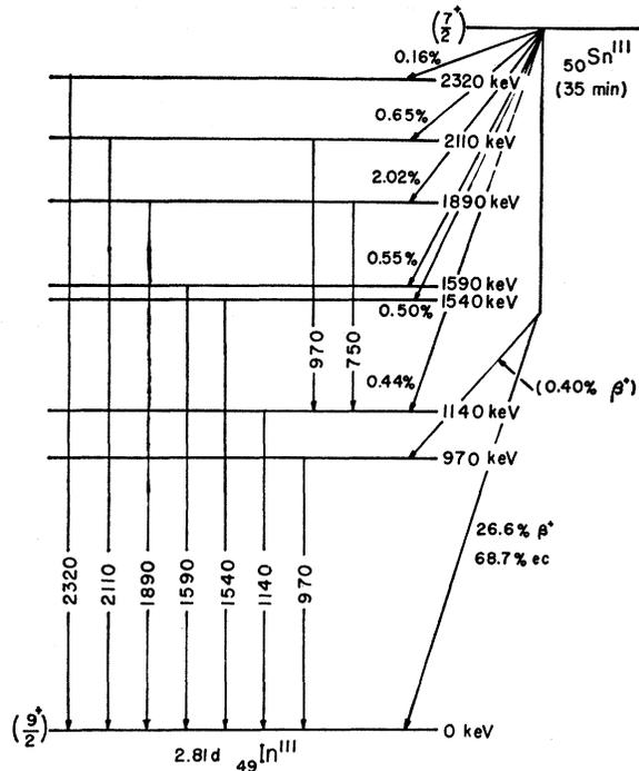
FIG. 8. Proposed decay scheme for  $\text{Sn}^{111}$ .
