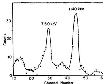
FIG. 5. Spectrum of gamma rays which are in coincidence and sum to form 1890-keV sum peak. The peaks are statistically of equal intensity.
