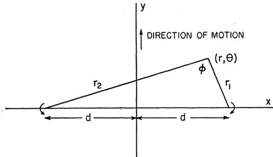
FIG. 2. The geometry of the vortex pair, showing the direction of motion and the sense of rotation.
