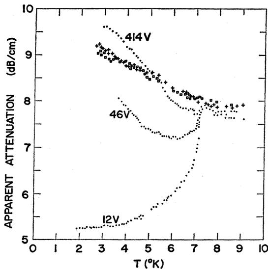
FIG. 8. Apparent attenuation (see text for discussion) versus temperature for various initial-pulse amplitudes. The 30-Mc/sec longitudinal pulse was propagated in the [111] direction. The curves labeled by transducer voltages are all in the superconducting state while the crosses (+) and squares ( $\square$ ) correspond to normal-state data with 12 and 414 V on the transducer, respectively. Some points near  $T_c$  have been omitted.
