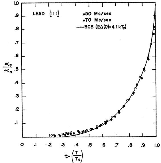
FIG. 3. Ratio of electronic attenuations versus reduced temperature for propagation in the  $[111]$  direction. The solid line illustrates the temperature dependence predicted by the BCS theory for the indicated zero-temperature energy gap.
