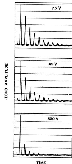
FIG. 7. Traces of oscilloscope photographs showing the detected echos as a function of time for the indicated peak-to-peak initial-pulse voltages at the transducer. A 30-Mc longitudinal pulse was being propagated in the [100] direction at 2.69°K.
