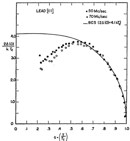
FIG. 5. Energy gap in units of  $kT_c$  derived from data of Fig. 3.
