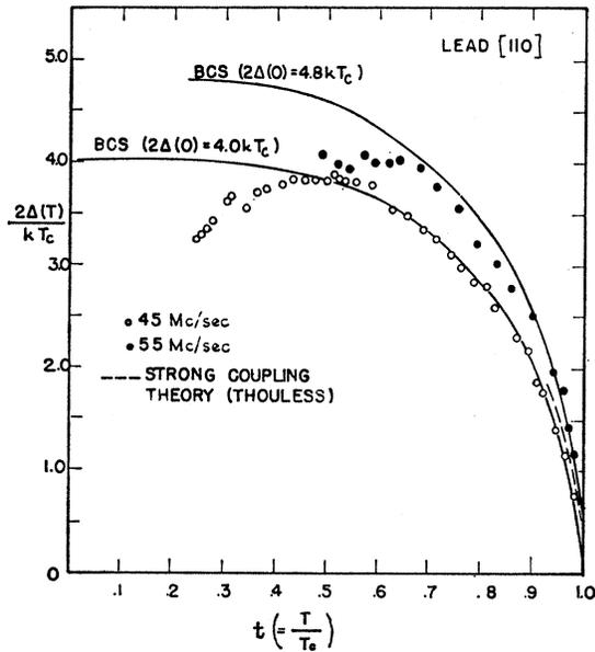
FIG. 6. Energy gap in units of  $kT_c$  derived from data of Fig. 4.
