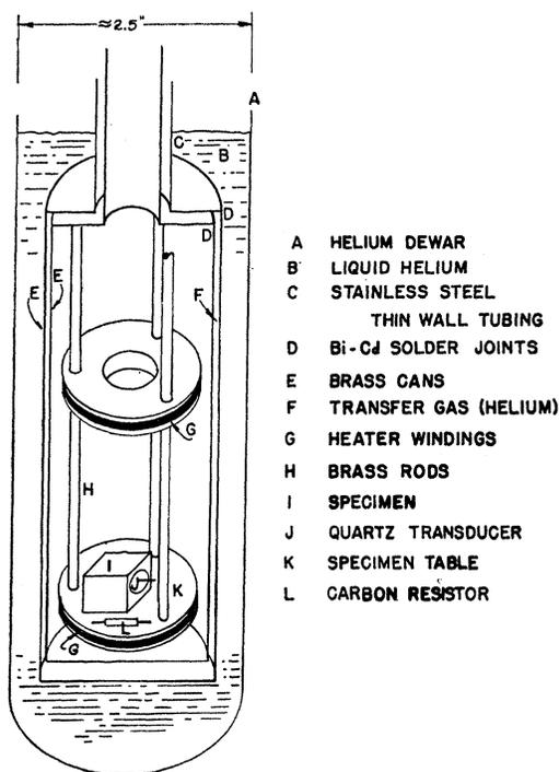
FIG. 1. Cutaway of specimen chamber.
