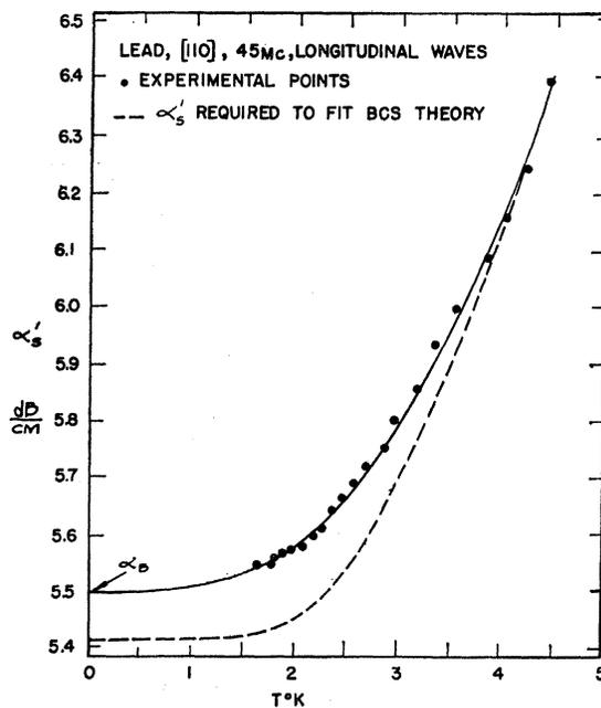
FIG. 9. Experimental  $\alpha'_s$  versus temperature. The dashed line was computed using BCS theory with a zero-temperature energy gap of  $4kT_c$  and experimental  $\alpha_n$  values.
