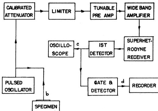
FIG. 2. Block diagram of circuitry for ultrasonic measurement.
