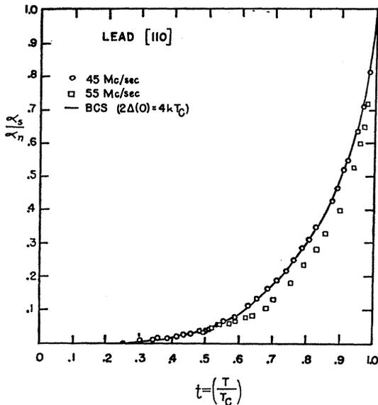
FIG. 4. Ratio of electronic attenuations versus reduced temperature for propagation in the [110] direction.
