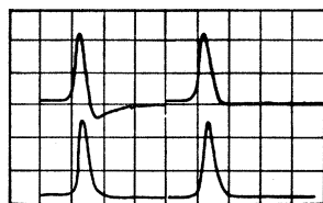
FIG. 6. Top: The effect of a magnetic field on the signal level. Bottom: Monitor of the laser intensity. The horizontal sweep is 10^{-7} sec/cm.
