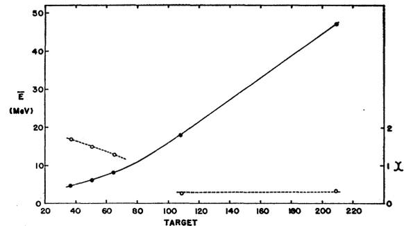
FIG. 5. Solid curve—variation with target  $A$  of the mean energy of  $\text{Na}^{24}$  emitted at  $90^\circ$  from 2.9-GeV proton irradiation of various targets. The ordinate scale at the left applies. Dashed curve variation with target  $A$  of the skewness coefficient  $\chi$  for the energy spectra of  $\text{Na}^{24}$ . The ordinate scale at the right applies. Data in this figure are from the present study and from Refs. 13 and 20.
