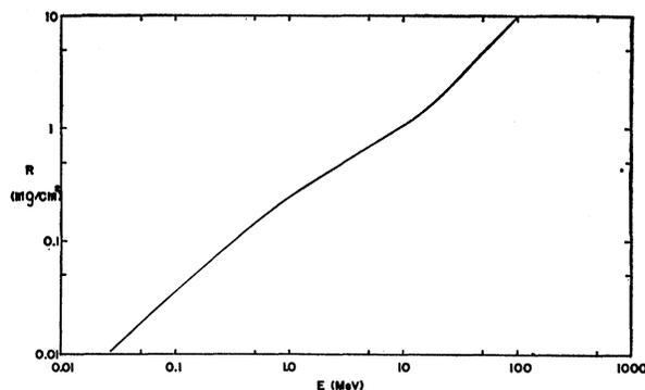
FIG. 3. Range-energy relation for Na<sup>24</sup> in Formvar.
