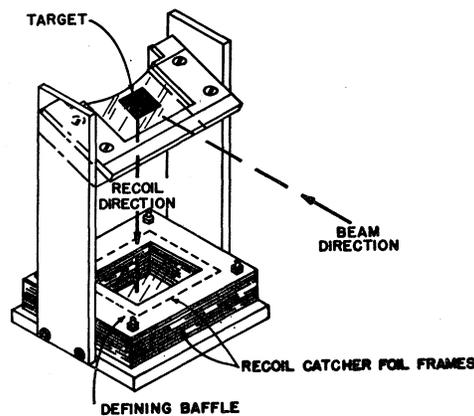
FIG. 1. Apparatus for measuring differential ranges at  $90^\circ$  to beam direction.
