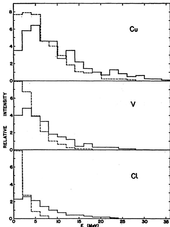
FIG. 6. Comparison of energy spectra for  $\text{Na}^{24}$  obtained from cascade-evaporation calculations (solid histograms) with those obtained from evaporation calculations (dashed histograms).
