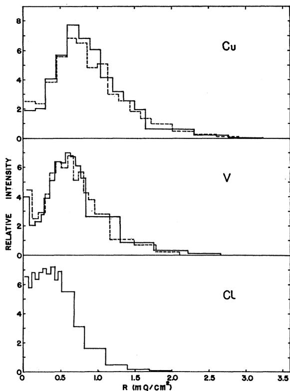
FIG. 2. Observed range distributions at 90° of Na<sup>24</sup> from 2.9-GeV proton irradiation of the indicated targets. The dashed histograms are the results of duplicate experiments with thicker targets normalized to the same area as the corresponding thin target histograms.
