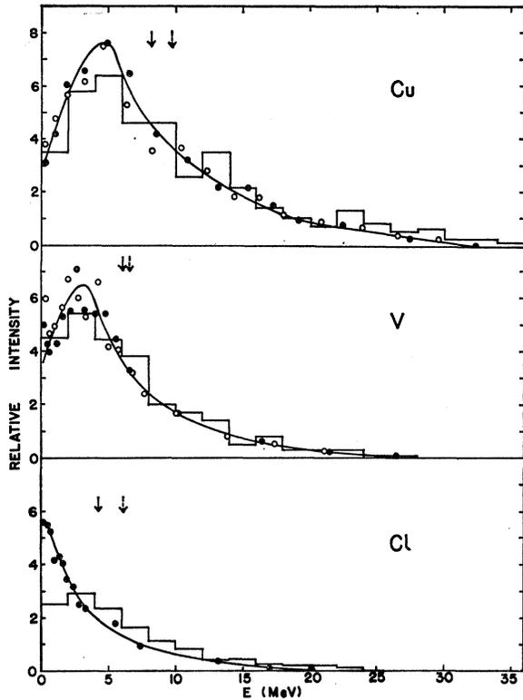
FIG. 4. Energy spectra at  $90^\circ$  of  $\text{Na}^{24}$  from 2.9-GeV proton irradiation of the indicated targets. Experimental data are shown by the points and the smooth curves through them. (Open points are the results of duplicate experiments with thicker targets.) The histograms show the results of the cascade-evaporation calculation. The solid and dashed arrows refer to mean experimental and calculated energies respectively.
