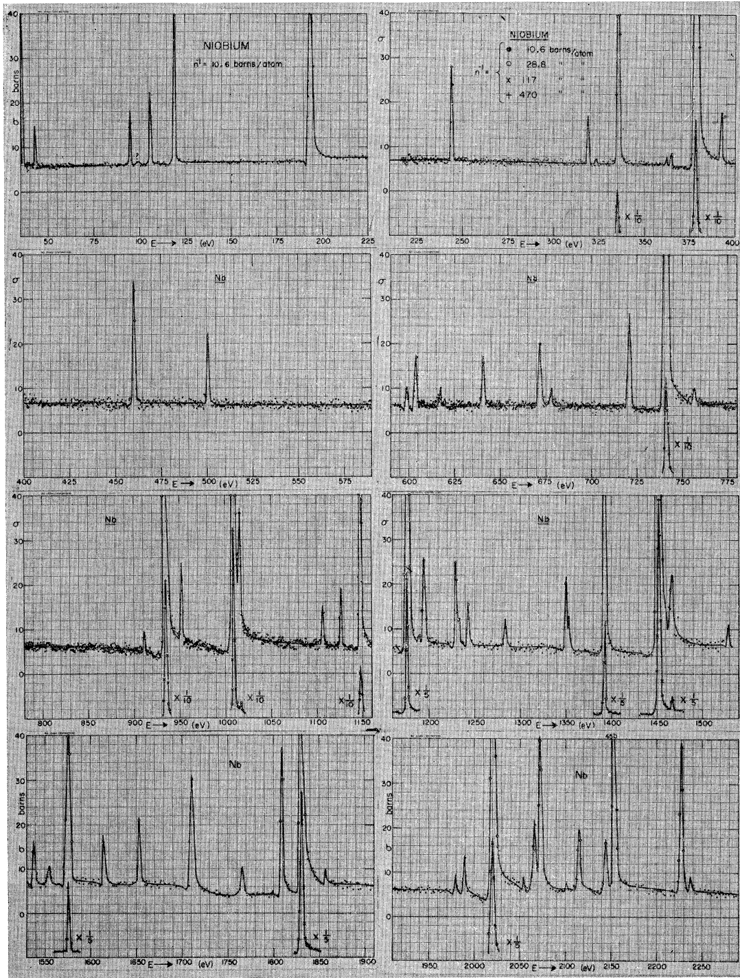
FIG. 1. The "measured" total neutron cross section of Nb^{93} versus energy from 35 to 7250 eV. The measurements used four sample thicknesses as indicated, with the cross section between resonances mainly determined from the thick-sample data. At resonance the data for progressively thinner samples was used. When the resonance cross section exceeds full-scale value an insert scale is shown having its zero start at the bottom of the page with a factor of 5, 10, or 20, as indicated reduction in the height of the curve. In the region of resonance the peak cross-section values are distorted by Doppler level broadening, the instrumental energy resolution, and by the (1/n) value for the thinnest sample. The cross-section values are in barns.
